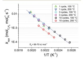
Fig. 3 Arrhenius plot for  $k_{\rm app}$  of propene oxidation over the Pt/GNP composites obtained after 1, 3, and 10 cycles at both 100 °C and 200 °C.
