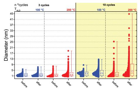
Fig. 4 Box-and-whisker plots and data overlap of the number-based size distributions of the Pt nanoparticles obtained after 3 and 10 cycles at both 100 °C and 200 °C before and after the catalytic test. The boxes indicate the 10th, 25th, 75th, and 90th percentiles of the population, the whiskers indicate the minimum and the maximum size, and the white diamonds indicate the average size.
