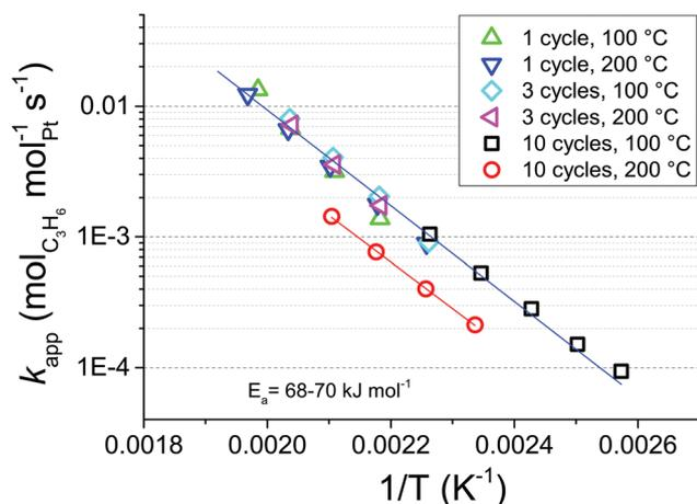
Fig. 3 Arrhenius plot for  $k_{app}$  of propene oxidation over the Pt/GNP composites obtained after 1, 3, and 10 cycles at both 100 °C and 200 °C.
