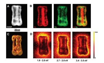
Fig. 6 Structural and electromagnetic characterization of an individual nanorattle. HAADF-STEM image of a nanorattle (A), STEM-EDS elemental maps revealing the distribution of Au and Ag in the structure (B) threedimensional (3D) representation of the reconstructed volume of the nanorattle shown in A, (C) revealing the lateral separation between inner core and shell. STEM-EELS mappings (D) at distinct energies show electric field enhancement inside of the cavity.
