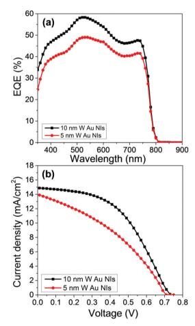
Fig. 3 (a) EQE action spectra and (b) device performance for NiO ultrathin films with thicknesses of 5 and 10 nm with Au NIs based on the device structure of ITO/NiO/PSK/PCBM/Ag.
