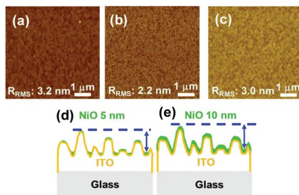
Fig. 4 AFM images of (a) bare ITO substrate, (b) 5 nm-thick NiO/ITO, and (c) 10 nm-thick NiO/ITO. The magnification is  $\times 12500$ , and the scale bar is  $1 \mu\text{m}$  for all AFM figures. Schematic of the two different thicknesses of NiO PLD thin films, (d) 5 nm and (e) 10 nm, showing their coverage and roughness on the ITO surface.
