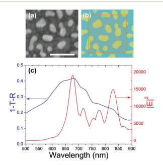
Fig. 6 The SEM image of Au NIs on the 10 nm-thick NiO film (a) and its corresponding model for FDTD numerical simulations (b). The scale bar in the SEM image is 100 nm. The inset color region of (b) is a simulation area on the x-y plane. (c) The 1-T-R spectrum and the action spectrum of near-field intensity monitored at the interface between Au NIs and the NiO film calculated by the FDTD numerical simulations.
