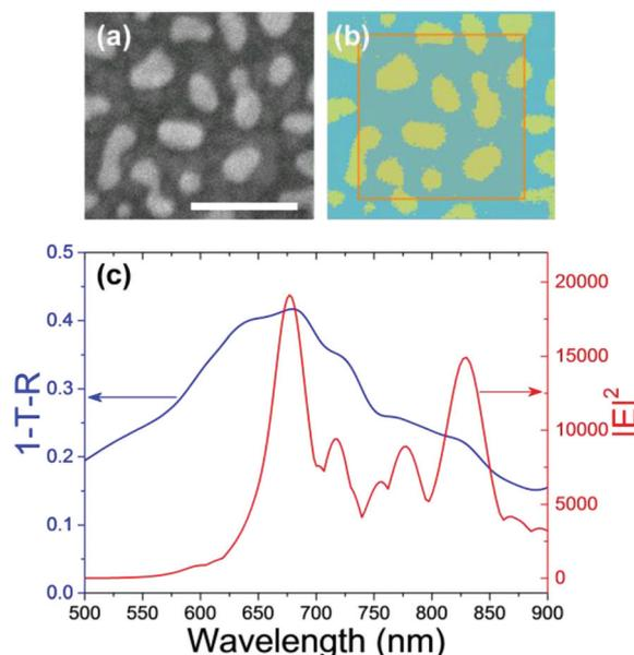
**Fig. 6** The SEM image of Au NIs on the 10 nm-thick NiO film (a) and its corresponding model for FDTD numerical simulations (b). The scale bar in the SEM image is 100 nm. The inset color region of (b) is a simulation area on the  $x$ – $y$  plane. (c) The 1-T-R spectrum and the action spectrum of near-field intensity monitored at the interface between Au NIs and the NiO film calculated by the FDTD numerical simulations.
