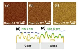
Fig. 4 AFM images of (a) bare ITO substrate, (b) 5 nm-thick NiO/ITO, and (c) 10 nm-thick NiO/ITO. The magnification is  $\times 12500$ , and the scale bar is 1  $\mu m$  for all AFM figures. Schematic of the two different thicknesses of NiO PLD thin films, (d) 5 nm and (e) 10 nm, showing their coverage and roughness on the ITO surface.
