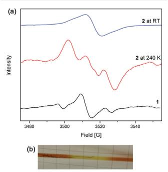
Fig. 3 (a) EPR spectra in  $[(n-C_4H_9)_4N]PF_6/CH_3CN$  electrolyte of **1** and **2** at 240 K and room temperature and (b) photo of the EPR cell with electrodes during the experiment showing the colour change from deep red to yellow.
