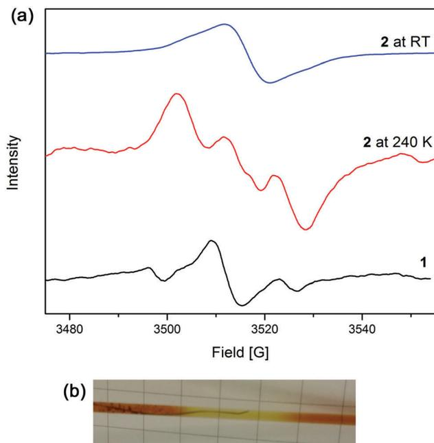
Fig. 3 (a) EPR spectra in  $[(n\text{-C}_4\text{H}_9)_4\text{N}]\text{PF}_6/\text{CH}_3\text{CN}$  electrolyte of **1** and **2** at  $240\text{ K}$  and room temperature and (b) photo of the EPR cell with electrodes during the experiment showing the colour change from deep red to yellow.
