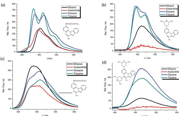
λ/nm λ/nm Fig. 2 Fluorescence emission spectra in ethanol, acetonitrile, dioxane and toluene at the concentration of  $1 \times 10^{-7}$  mol dm<sup>-3</sup> of 3 (a), 4 (b), 5 (c) and 6
