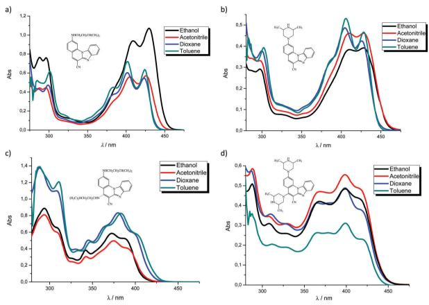
Fig. 1 UV-Vis spectra recorded in ethanol, acetonitrile, dioxane and toluene at concentrations of  $2 \times 10^{-5}$  mol dm<sup>-3</sup> of **3** (a), **4** (b), **5** (c) and **6** (d).
