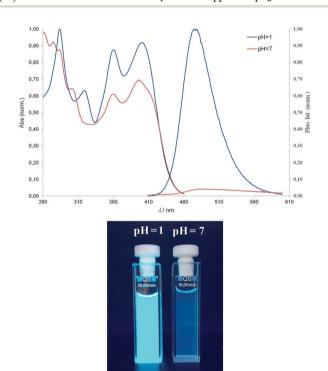
Fig. 3 Typical absorption and fluorescence emission spectra of compound **6** ( $\lambda_{\text{exc.}} = 397 \text{ nm}$ ) in buffer at pH = 7 and pH = 1 (bottom).
