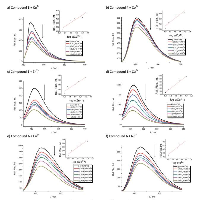
Fig. 6 Fluorimetric titrations of compound 3 with Zn<sup>2+</sup> (a), 4 with Co<sup>2+</sup> (b), 5 with Zn<sup>2+</sup> (c) and Cu<sup>2+</sup> (d) and 6 with Co<sup>2+</sup> (e) and Ni<sup>2+</sup> cations (f). The insets show approximately linear decrease in fluorescence intensity with the logarithm of the metal concentration.
