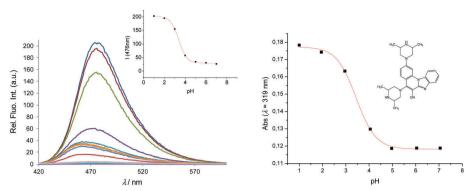
Fig. 4 Fluorescence emission spectra of  $\bf 6$ ,  $2 \times 10^{-6}$  mol dm<sup>-3</sup> at different pH values (left) and its calibration curve (right); absorbance versus pH at 319 nm
