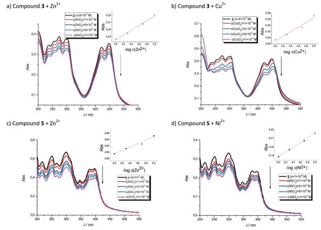
Fig. 5 UV-Vis titrations of compound 3 with Zn<sup>2+</sup> (a) and Cu<sup>2+</sup> cations (b) and titrations of compound 5 with Zn<sup>2+</sup> (c) and Ni<sup>2+</sup> cations (d). The insets show approximately linear decrease in absorption with the logarithm of the metal concentration.
