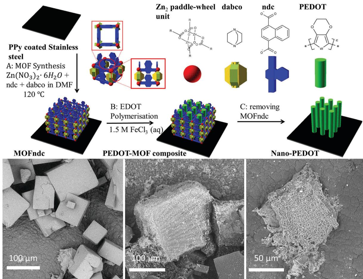
**Fig. 1** Schematic diagrams illustrate the experimental steps in sequence: synthesis of MOFndc on PPy coated stainless steel, chemical polymerisation of EDOT in MOFndc, and formation of nano-PEDOT after removing PEDOT. SEM images obtained with back-scattered electrons (BSE) reveal the morphologies of the products at the steps A–C. 3D schematics are created with open sourced software available from <http://www.openscad.org/>.
