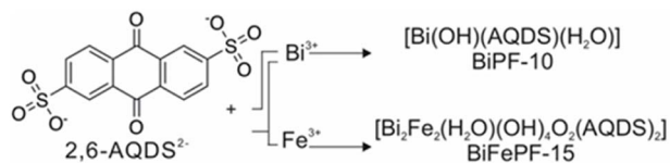
Scheme 1 Single- and bimetal MOFs have been synthesized with the same anthraquinone based linker.
