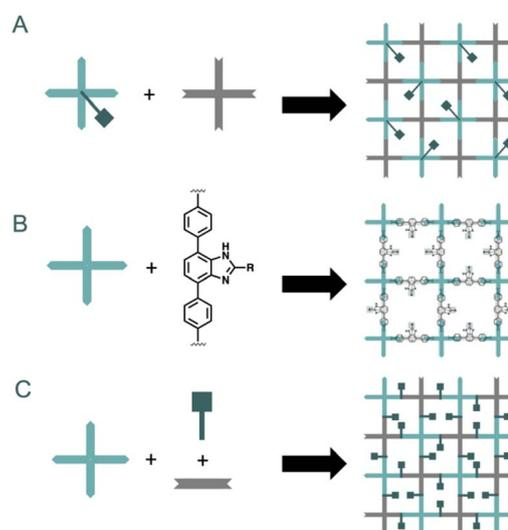
Fig. 9 Different strategies for *de novo* construction of COFs: incorporation of a functionalizable moiety in a well-known core (A), incorporation of 4,7-disubstituted benzimidazole as building block core (B), assembly of the network using a multicomponent reaction (C).
