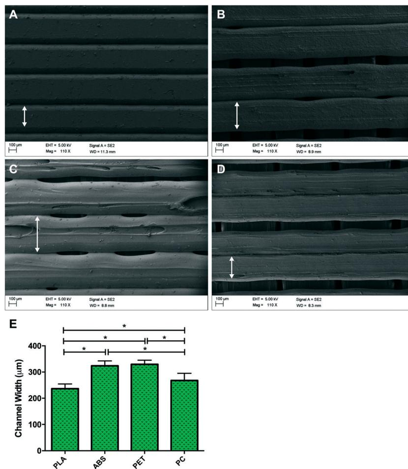
**Fig. 2** SEM images for (A) polylactic acid (PLA), (B) acrylonitrile butadiene styrene (ABS), (C) polyethylene terephthalate (PET) and (D) polycarbonate (PC) 3D-printed polymers *via* FDM. Arrows indicate central raised plateau of channel on each polymer. (E) Channel widths of PLA, ABS, PET and PC 3D-printed polymers *via* FDM. Data presented as mean  $\pm$  SD from  $n = 3$  discs per polymer. \* one-way ANOVA/non-parametric equivalent  $P \leq 0.05$ . Scale bars = 100  $\mu\text{m}$ .
