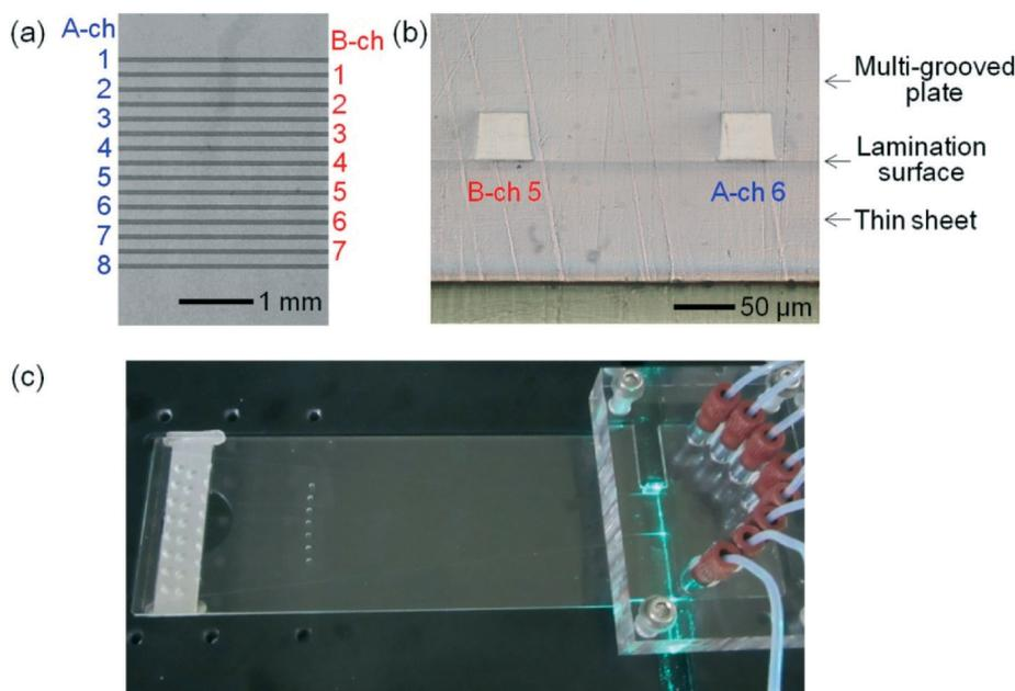
**Fig. 2** Photographs of the fabricated multi-channel microchip. (a) Top view of the microchip around the laser-irradiation region showing eight A channels and seven B channels. (b) Cross-sectional view of the microchip around the laser-irradiation region showing B-ch 5 and A-ch 6. (c) The microchip on an optical stage with the side-entry laser beam and the polymer filling unit.
