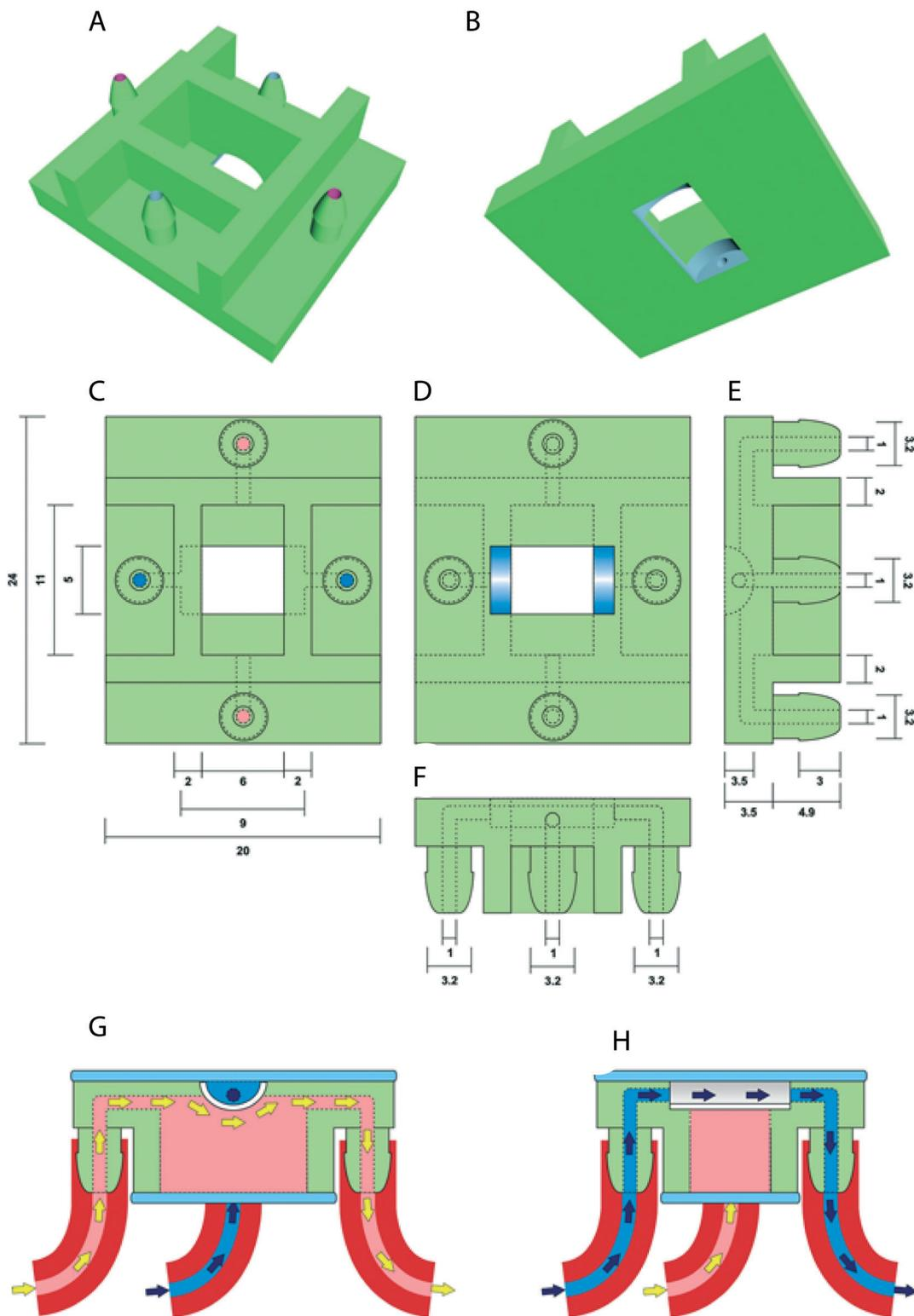
**Fig. 1** Perspective visualization of the open device's 3D printable model from above (A) and below (B). Schematic top (C), bottom (D), right (E) and front (F) view of the open device. Schematic right (G) and front (H) cross section of the closed device while being separately perfused with two (pink and blue) different types of media/cells. Dimensions are represented in millimeters.
