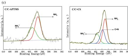
Fig. 4 Surface chemical composition of the pristine and functionalized C/C: (a) XPS wide spectra, (b) high-resolution spectra of carbon peaks ( $C_{1s}$ ) and the relative content of functional groups of C/C-OH, C/C-APTMS and C/C + CS, (c) high-resolution spectra of nitrogen peak ( $N_{1s}$ ) for C/C-APTMS and C/C + CS.
