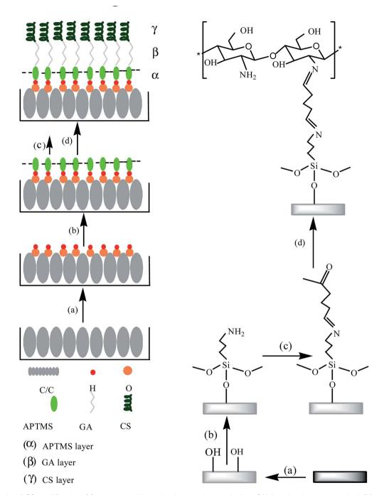
Fig. 1 Schematic of CS modification: (a) treatment with a piranha solution to obtain -OH functional group terminal, (b) polycondensation reaction of APTMS molecule and -OH group of the C/C top surface, (c) silane coupling reaction of glutaraldehyde and APTMS, (d) covalent grafting of CS onto the APTMS molecular architecture.
