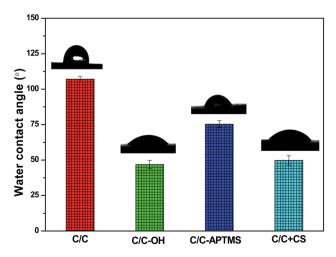
Fig. 3 Water contact angle of different C/C samples.
