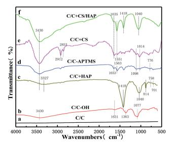
Fig. 5 FTIR spectra of C/C, C/C-OH, C/C + HAP, C/C-APTMS, C/C + CS and C/C + CS/HAP samples.
