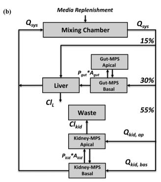
Fig. 1 Schematic overview of (a) a gut-liver-mixing chamber platform (multi-MPS platform I) and (b) a gut-liver-kidney-mixing chamber platform (multi-MPS platform II). Three scaling approaches were investigated to determine design (i.e. model) parameters and checked for their feasibility to satisfy the study objective.  $Q_{sys}$  = systemic flow rate,  $Q_{kid}$  = flow rate to kidney,  $P_i$  = permeability,  $A_i$  = surface area,  $Cl_i$  = clearance; L = liver, kid = kidney.
