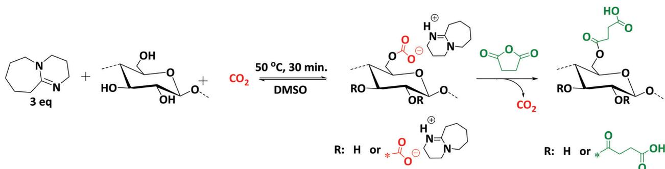
**Scheme 2** Dissolution and activation of cellulose for the subsequent derivatization with succinic anhydride using CO<sub>2</sub>-based switchable solvent.
