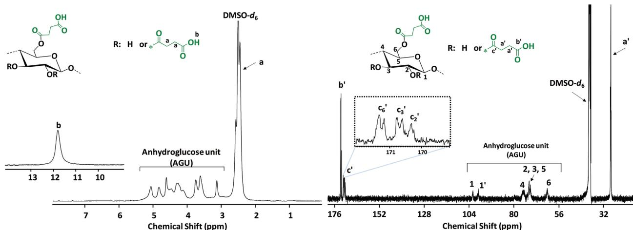
Fig. 2 <sup>1</sup>H (left) and <sup>13</sup>C NMR (right) of the succinylated filter paper (SFP 6) in DMSO-*d*<sub>6</sub>.
