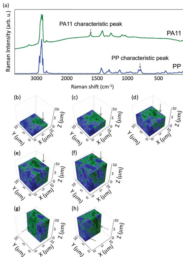
**Fig. 4** (a) Raman spectra for PP and PA11 resins and (b–h) three-dimensional analytical results for sample #8 (bottom). Legend for (b–h): blue, PP; green, PA11; arrows and broken arrows indicate PP and PA11, respectively. The measurement regions were  $10 \times 10 \times 10 \mu\text{m}$ . Observed faces (in  $\mu\text{m}$ ): (b)  $z = 0.3$ , (c)  $z = 2.7$ , (d)  $z = 5.1$ , (e)  $z = 7.5$ , (f)  $z = 9.9$ , (g)  $x = 5.0$ , and (h)  $y = 5.0$ .
