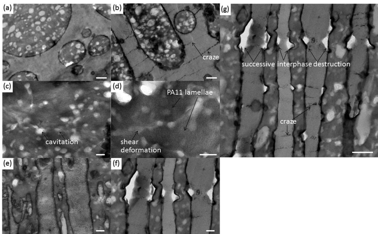
Fig. 5 TEM images of sample #8 stained with OsO<sub>4</sub> and RuO<sub>4</sub>. (a, e) Before and (b–d, f, g) after the Charpy notched impact strength test. The scale bar represents 500 nm for (a, b, g) and 200 nm for (c–f).
