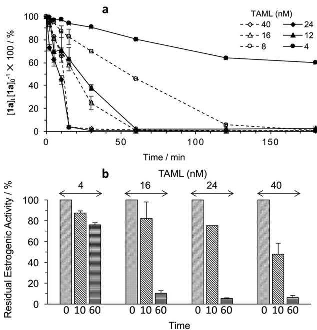
Fig. 7 (a) Kinetic traces of **2** (concentrations shown) catalysed oxidation of **1a** (43.8  $\mu\text{M}$ ) by H<sub>2</sub>O<sub>2</sub> (4 mM) at pH 8.5 (0.01 M, carbonate) and 25 °C. Data points are each the mean of triplicate runs with estimated 3SD limits indicated. (b) Residual oestrogenic activity as a function of treatment time for some of the processes shown in (a).
