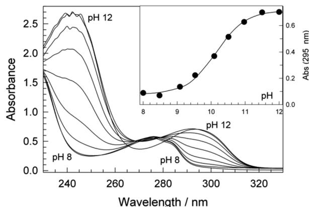
Fig. 4 UV-vis variation with pH for **1a**. Inset shows absorbance changes at 295 nm as a function of pH; the solid line is the calculated dependence using the best-fit values of eqn (1). Conditions:  $[1a] 1.5 \times 10^{-5}$  M, 25 °C, 0.01 M phosphate.
