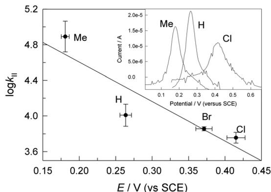
Fig. 6 Relationship between  $\log k_{\text{II}}$  and experimentally determined reduction potentials of **1** obtained by differential pulse voltammetry in acetonitrile (Inset) of solutions of **1** ( $[\mathbf{1}] \approx 10^{-3}$  M). Conditions: 0.1 M  $[\text{n-Bu}_4\text{N}]\text{PF}_6$  as supporting electrolyte, modulation time 0.05 s, interval time 0.1 s, step potential 0.002 V, modulation amplitude 0.005 V, scan rate  $0.1 \text{ V s}^{-1}$ , glassy carbon electrode.
