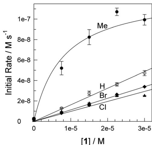
Fig. 5 Dependence of the initial rate of oxidation of substituted Bisphenol A derivatives **1a–d** (**1**: a = H, b = Me, c = Cl, d = Br) by H<sub>2</sub>O<sub>2</sub> ( $7.5 \times 10^{-3}$  M) catalysed by **2** ( $1.5 \times 10^{-7}$  M). Conditions: 0.01 M phosphate ( $\text{Na}_2\text{HPO}_4$ ), pH 11, 25 °C.
