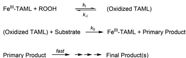
Scheme 1 Stoichiometric mechanism of catalysis by TAML/peroxide.
