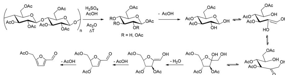
Scheme 1 Proposed reaction mechanism for AMF formation.
