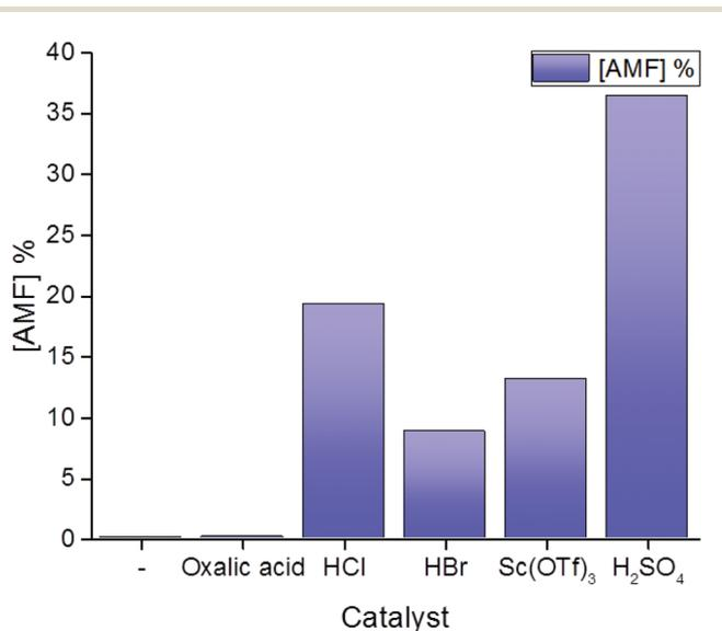
**Fig. 1** AMF yield for the acetolysis of cellulose acetate in the presence of different catalysts. General conditions: cellulose acetate, acetic anhydride, catalyst, 200 °C, 2 hours. For details of the reaction conditions please refer to the ESI.†
