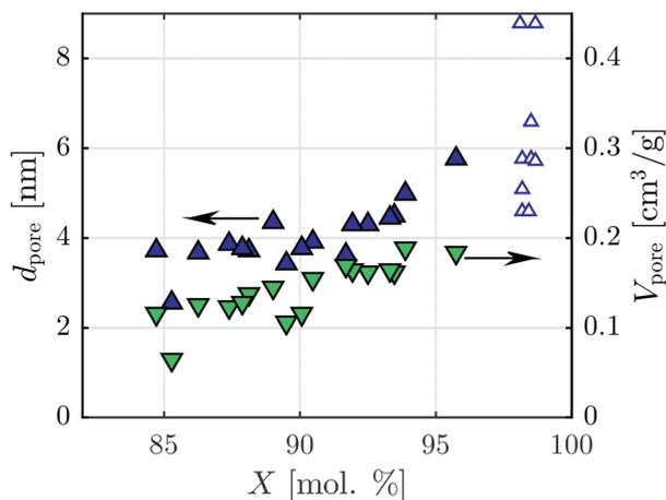
**Fig. 10** Mean pore diameter,  $d_{\text{pore}}$ , and total specific pore volume,  $V_{\text{pore}}$ , of the solar-produced aluminas as a function of the extent of chemical conversion,  $X$ , for experimental runs 1 to 17. Also shown with open symbols are the typical mean pore diameter of nine SGAs produced with industrial calciners as reported in the literature.<sup>28,32,34</sup>
