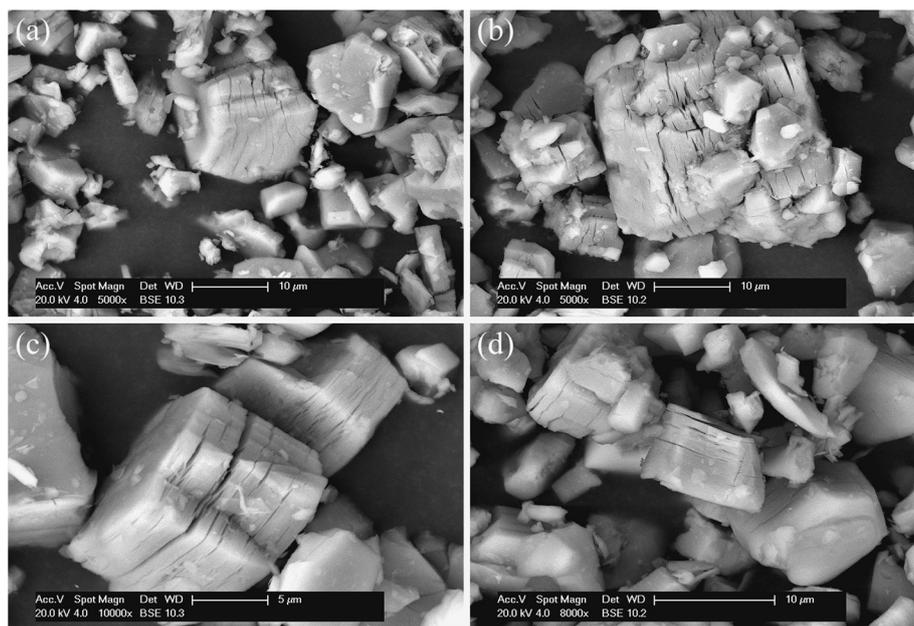
**Fig. 9** SEM micrographs of solar-processed alumina obtained from experimental runs (a) #4 ( $T_{\text{wall}} = 934$  K), (b) #11 ( $T_{\text{wall}} = 1311$  K), (c) #14 ( $T_{\text{wall}} = 1371$  K), and (d) #19 ( $T_{\text{wall}} = 1262$  K) at 5000, 5000, 10 000, and 8000 magnification, respectively.
