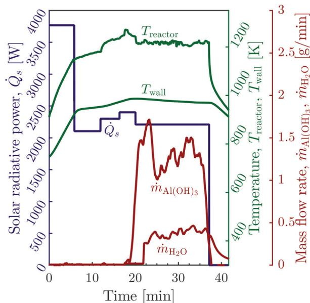
**Fig. 5** Temporal variations of solar radiative power input,  $\dot{Q}_s$ , reactor temperatures,  $T_{\text{reactor}}$  and  $T_{\text{wall}}$ , particle mass feed rate,  $\dot{m}_{\text{Al}(\text{OH})_3}$ , and mass flow rate of evolved water within the outlet stream,  $\dot{m}_{\text{H}_2\text{O}}$ , during a representative solar experimental run (#9).
