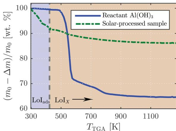
**Fig. 4** Relative mass change of the reactant  $\text{Al}(\text{OH})_3$  and a representative solar-processed alumina as a function of the reference TGA temperature,  $T_{\text{TGA}}$ , during a dynamic TGA run between 298 K and 1273 K in synthetic air. The temperature ranges used in the present study for determining  $\text{LoI}_{\text{ads}}$  and  $\text{LoI}_X$  are indicated.
