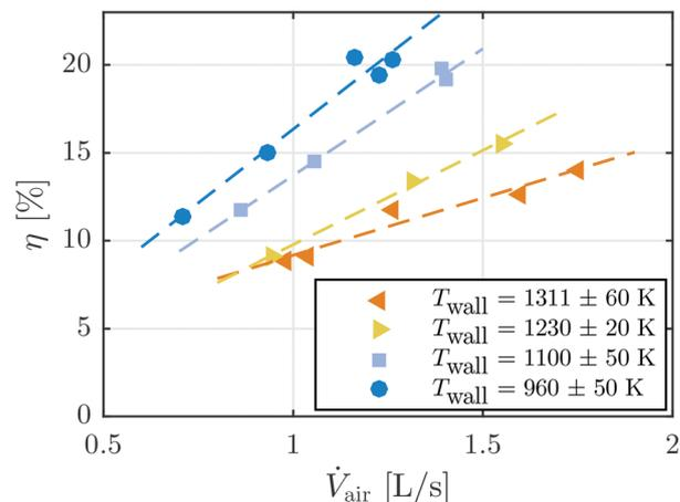
Fig. 7 The energy efficiency,  $\eta$  (defined in eqn (5)), of the present solar calcination reactor as a function of the volumetric flow rate of transport air,  $\dot{V}_{\text{air}}$ , for four different wall temperatures,  $T_{\text{wall}}$ . See Table 1 for details.
