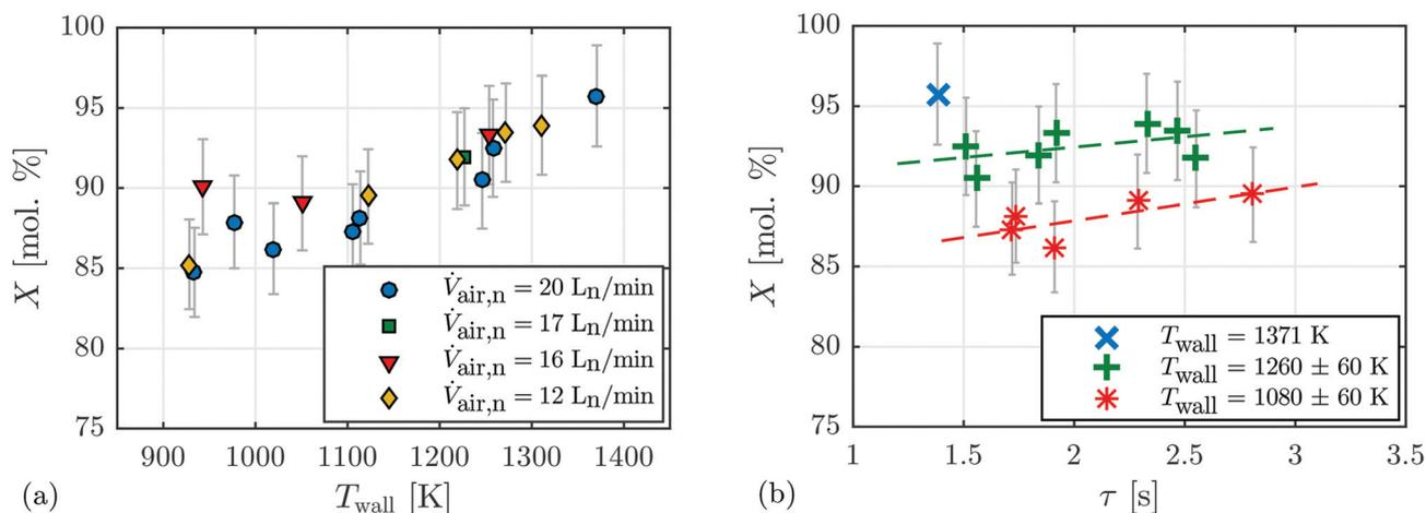
Fig. 6 The extent of chemical conversion,  $X$ , as a function of (a) the average characteristic wall temperature,  $T_{\text{wall}}$ , for four different air normal flow rates,  $\dot{V}_{\text{air},n}$ , and for experimental runs 1 to 17; and (b) the nominal particle residence time,  $\tau$ , for three different average characteristic wall temperatures,  $T_{\text{wall}}$ . Also shown are the linear lines of best fit for the data points in the two temperature ranges.
