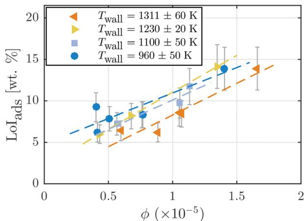
**Fig. 8** Mass percentage of adsorbed moisture,  $LoI_{ads}$ , in the product from the solar reactor as a function of the particle to air volume fraction,  $\phi$  (defined in eqn (3)), for four different wall temperatures,  $T_{wall}$ , for experimental runs 1 to 17.
