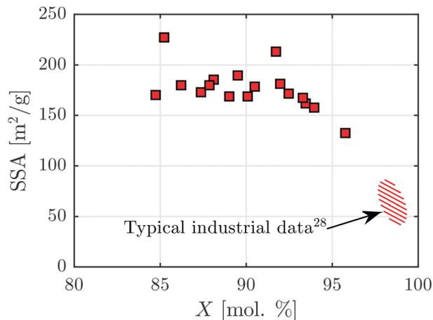
**Fig. 11** Specific surface area, SSA, of the present solar-produced aluminas as a function of the extent of chemical conversion,  $X$ , for experimental runs 1 to 17. Also shown is the typical  $X$  and SSA product quality properties of SGA calcined in an industrial gas suspension calciner.<sup>28</sup>
