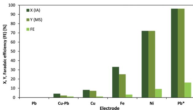
Fig. 2 Screening of various metal electrodes in the ECH of IA to MS. Conditions: r.t., 1 h, counter electrode: glassy carbon,  $E = -1.06$  V *vs.* standard-hydrogen-electrode (SHE), water (16 mL), H<sub>2</sub>SO<sub>4</sub> (0.5 mol L<sup>-1</sup>), IA (0.1 mol L<sup>-1</sup>, 1.6 mmol, 0.208 g). \* $E = -1.41$  V *vs.* SHE (X denotes conversion, Y means yield).
