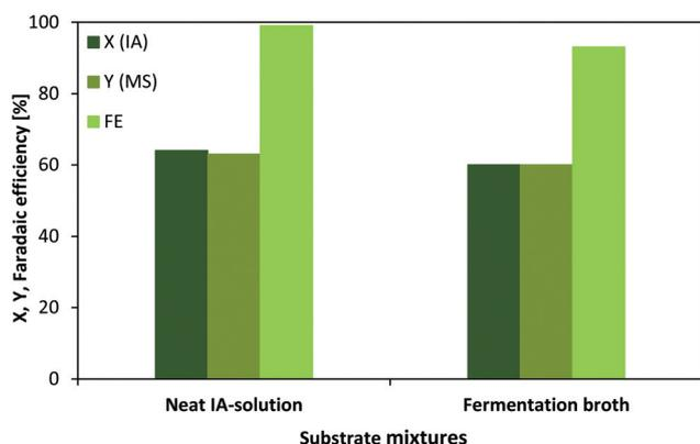
Fig. 4 Comparison of neat IA-solution with fermentation broth using Pb as WE. Conditions: r.t., 1 h, counter electrode: glassy carbon,  $i = 0.3 \text{ A}$ , neat IA-solution: water (16 mL),  $\text{H}_2\text{SO}_4$  ( $0.5 \text{ mol L}^{-1}$ ), IA ( $0.57 \text{ mol L}^{-1}$ , 9.1 mmol, 1.187 g).
