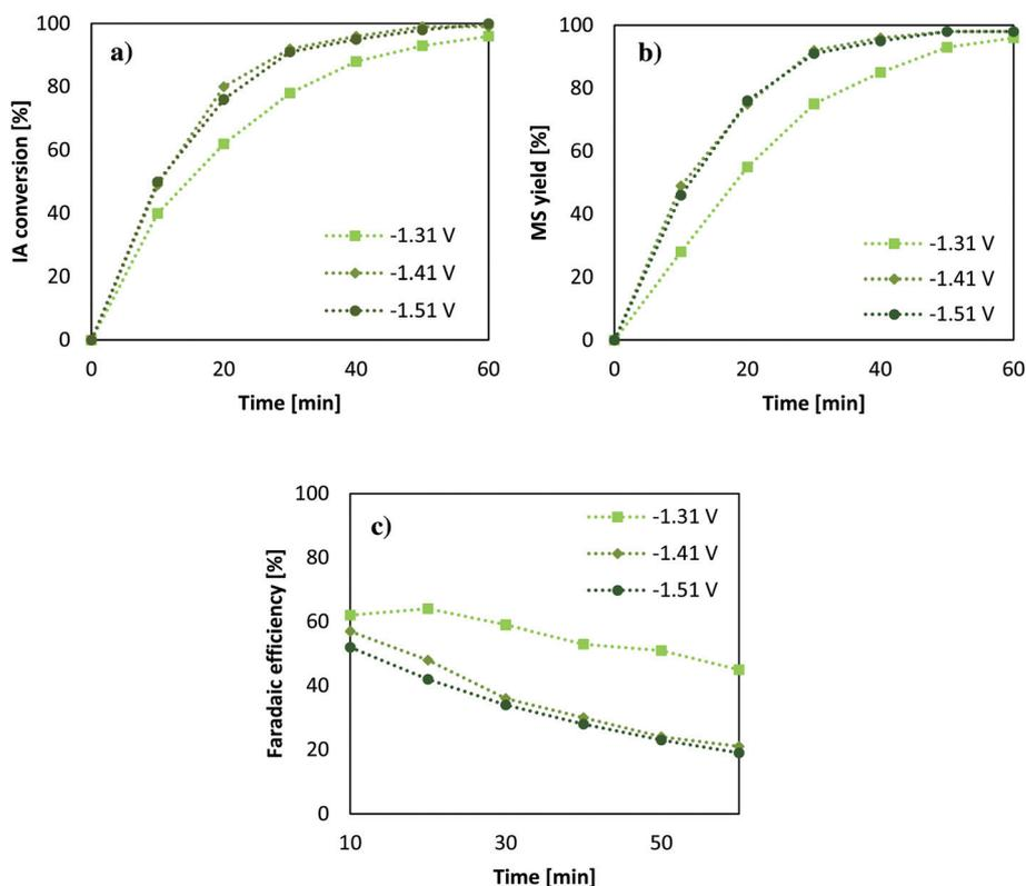
**Fig. 3** The effect of the applied potential on the conversion, yield and faradaic efficiency: (a) IA conversion, (b) yield of MS, and (c) faradaic efficiency. Conditions: r.t., working electrode: Pb, counter electrode: glassy carbon, water (16 mL),  $\text{H}_2\text{SO}_4$  ( $0.5 \text{ mol L}^{-1}$ ), IA ( $0.1 \text{ mol L}^{-1}$ , 1.6 mmol, 0.208 g). The dashed lines are added as guide to the eye.
