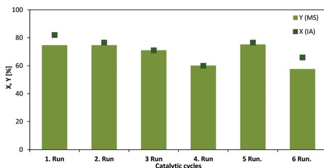
Fig. 5 Chemo-catalytic batch hydrogenation of IA over a Ru/C catalyst including recycling: 100 mg Ru/C in pure IA solution ( $0.61 \text{ mol L}^{-1}$ , 9.1 mmol, 1.187 g). Reaction conditions: 1 h,  $70 \text{ }^\circ\text{C}$ , 10 bar of  $\text{H}_2$ , 15 mL water, 500 rpm stirring speed.
