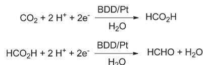
**Scheme 8** Electrocatalytic reduction with boron doped-diamond electrodes with highest efficiency for formaldehyde at -1.7 V.<sup>16</sup>
