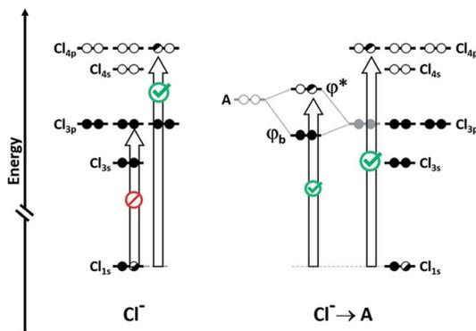
Fig. 6  $Cl_{1s}$  to  $Cl_{3p}$  transition, which can be probed by XAS, arises only if  $Cl_{3p}$  to  $I_2(\sigma^*)$  charge-transfer is present (A represents a halogen-bond acceptor, here  $I_2$ ). The intensity of the transition is proportional to the  $Cl_{3p}$  character in the  $\psi^*$  orbital. Reproduced from DOI: 10.1039/c7fd00076f with permission from The Royal Society of Chemistry.
