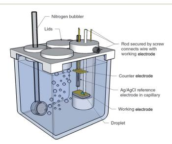
Fig. 1 Experimental cell and configuration used to obtain the liquid—liquid electrowetting measurements. The size of the glass cuvette is 5 cm  $\times$  5 cm  $\times$  5 cm.
