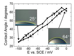
Fig. 2 Electrowetting response for a dichloroethane droplet on mercury surrounded by  $0.10 \text{ mol dm}^{-3} \text{ LiCl.}$
