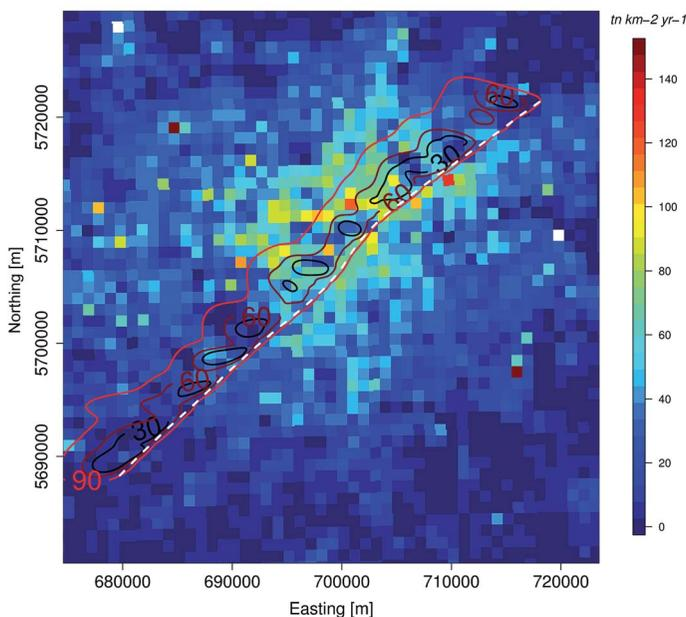
Fig. 5 Example footprint for 2014 RF transect over London showing the 30, 60, 90% footprint influence areas from the flight track (white), overlaid onto  $1 \text{ km}^2$  NAEI total NMHC emission estimates.
