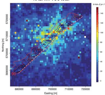
Fig. 5 Example footprint for 2014 RF transect over London showing the 30, 60, 90% footprint influence areas from the flight track (white), overlaid onto 1 km<sup>2</sup> NAEI total NMHC emission estimates.
