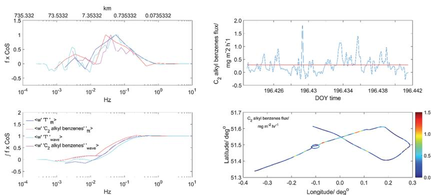
Fig. 2 Co- and cumulative co-spectra of wavelet (wT) and FFT C<sub>2</sub> alkyl benzenes and temperature fluxes.
