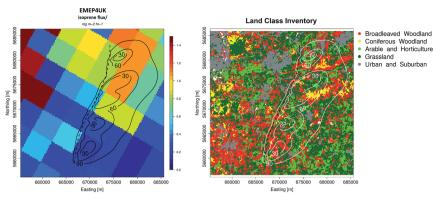
Fig. 7 RF flight track during a 2013 flight over the South Sussex region. (Left) Calculated footprint extent 30, 60, and 90% from flight track, overlaid onto EMEP4UK isoprene emission grid. (Right) Footprint extent 30, 60, and 90% from flight track, overlaid onto UK National Land Class Inventory 2012 at 25 m<sup>2</sup> resolution.
