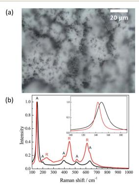
Fig. 1 (a) Micrograph of an illuminated UV100 sample surface ( $50 \times$  magnification). (b) Normalized Raman spectra of the illuminated UV100 sample: (black) white area and (red) dark area (exposed to the laser beam with a laser intensity of  $10 \times 50$  mJ cm<sup>-2</sup> per pulse).
