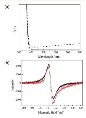
Fig. 2 (a) UV-vis diffuse reflectance spectra of (solid) untreated and (dash) illuminated UV100. (b) EPR spectra measured at 77 K of (black) illuminated UV100  $\text{TiO}_2$  anatase and (red) illuminated R15  $\text{TiO}_2$  rutile (exposed to the laser beam with laser intensity: 10  $\times$  50 mJ cm<sup>-2</sup> per pulse).
