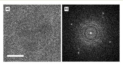
Fig. 5 (a) Cobalt nanoparticle inside the nanoreactor, at 1 bar  $N_2$  and 300 °C. Scale bar is 5 nm. (b) FFT of the image.
