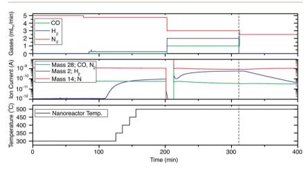
Fig. 4 Gas feed profile (top), QMS analyser data (middle), and nanoreactor temperature course (bottom) during the experiment. t=0 is indicated by the vertical dashed line.
