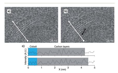
Fig. 7 Growth of a new carbon layer, indicated by the black arrows, interlayered between the cobalt surface and the set of carbon layers capping the nanoparticle, before (a) and after (b) the formation. Profiles of the white lines are shown in (c). Top profile: image (a); bottom profile: image (b). White line length is 5 nm.
