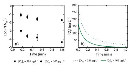
Fig. 7 At 22 °C (a) the effect of HRT on L. pneumophila inactivation, at two initial ozone concentrations and a WOM loading of 3.1 mg C L<sup>-1</sup> in a semi-batch reactor; (b) the profile of two initial dissolved ozone concentrations as a function of HRT. The data plotted in (a) are average values and standard deviations of three replicates. The dashed and solid curves in (b) are the results of calculations.
