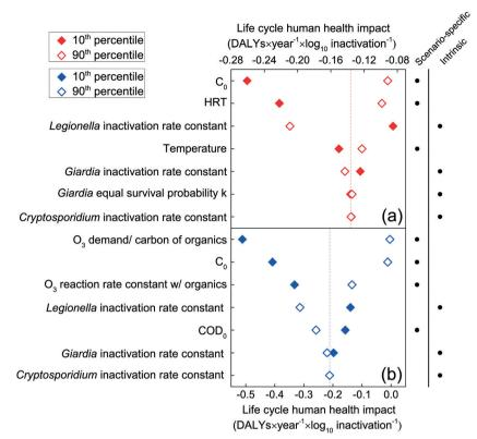
Fig. 5 The top seven input parameters to which human health impacts are most sensitive, for chlorination (a) and microplasma ozonation (b), expressed in DALYs × year 1 × log<sub>10</sub> pathogen inactivated 1. Sensitivity analysis for the rest of the parameters can be found in Fig. S4a and b in the ESI.†
