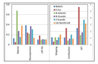
Fig. 5 Mean contribution to the  $PM_{2.5}$  concentration ( $\mu g \ m^{-3}$ ) per source and transport cluster from 22 September 2008 to 24 September 2009 in Gothenburg, Sweden. Note the different scales on the left and right hand side of the graph.
