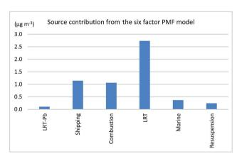
Fig. 2 Mean source contributions from the six-factor PMF model to the yearly mean PM<sub>2.5</sub> concentration.
