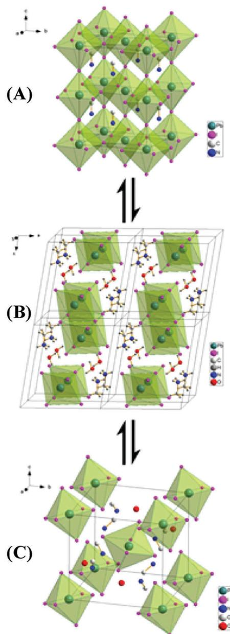
Fig. 13 (A) Structure of  $\text{MAPbI}_3$  in its cubic phase. (B) Structure of the monohydrate phase,  $\text{MAPbI}_3 \cdot \text{H}_2\text{O}$ . (C) Structure of the dihydrate,  $\text{MA}_4\text{PbI}_6 \cdot 2\text{H}_2\text{O}$ . Adapted from ref. 94, Copyright 2015 American Chemical Society.
