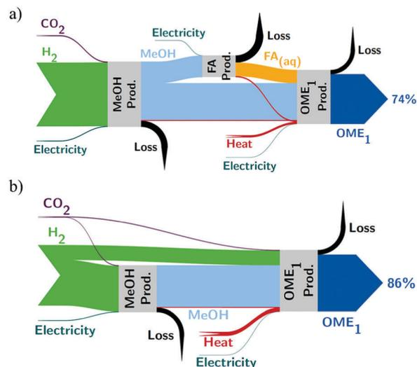
Fig. 3 Sankey diagram showing exergy flows in (a) the FA and (b) the direct route.
