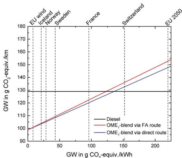
Fig. 8 Sensitivity analysis of the cradle-to-grave global warming (GW) impact of the OME<sub>1</sub>-blend and diesel fuel as a function of the GW impact of the electricity supply. The dashed vertical lines represent the GW impact of various national electricity grid mixes and a forecast average grid mix for Europe in 2050. CO<sub>2</sub> is supplied from a biogas plant.
