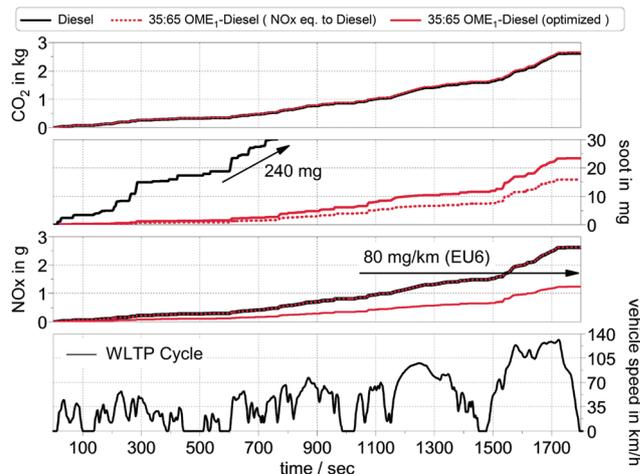
Fig. 5 Cumulative emissions of CO<sub>2</sub>, NO<sub>x</sub> and soot simulated over the Worldwide Harmonized Light Vehicles Test Procedures (WLTP) cycle. For the OME<sub>1</sub>-blend, two calibrations of the engine were used: the conventional diesel calibration (NO<sub>x</sub> eq. to diesel) and a variant optimized for low emissions, fuel consumption and combustion noise level (optimized).
