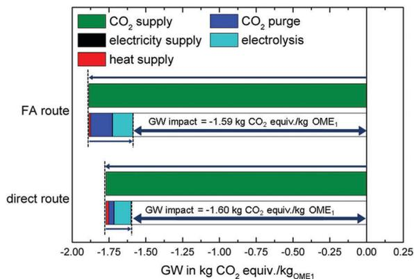
Fig. 2 Global warming (GW) impact from cradle-to-gate for the direct route and the FA route of  $\text{OME}_1$  for the best-case scenario. The green bars denote the negative GW impact of the  $\text{CO}_2$  supply captured from a biogas plant and thus avoiding emissions. The black, blue and cyan bars represent the positive GW impacts from the production of  $\text{OME}_1$ . The dark blue arrows represent the resulting total GW impact which is negative for both production routes.
