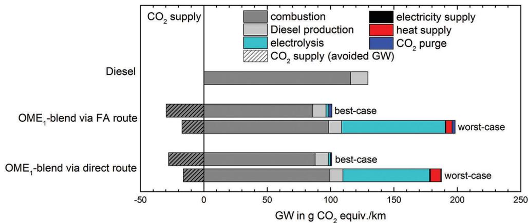
Fig. 7 Cradle-to-grave analysis of the global warming (GW) impact of the OME<sub>1</sub>-blend and fossil diesel fuel for the best- and the worst-case scenario specified in Table 3.
