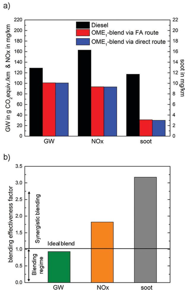
Fig. 6 (a) Cradle-to-grave analysis LCA results of the OME<sub>1</sub>-blend with the optimized calibration and fossil diesel fuel for the best-case scenario. (b) Blending effectiveness factor (BEF) (eqn (3)) of the OME<sub>1</sub>-blend for the global warming (GW) impact, and the emissions of NOx and soot for the best-case case scenario and the optimized engine calibration.
