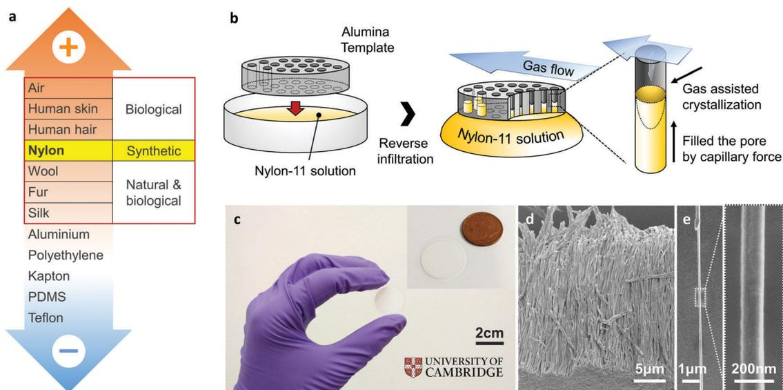
**Fig. 1** (a) Triboelectric series of common materials with highlighted position of tribo-positive materials. (b) Schematic of the nanowire fabrication procedure. (c) Photographs of a fabricated nanowire-filled AAO template. The inset shows size comparison with a British one-pence coin. (d and e) SEM images of template-freed nanowires and a single strand of Nylon nanowire, respectively.
