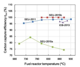
Fig. 7 Carbon capture efficiency comparison as a function of fuel reactor temperature for the different cases.
