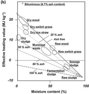
Fig. 2 (a) van Krevelen diagram for various fuels. Adapted from ref. 38 and 39. (b) Effect of moisture and ash content on the effective heating values of various biomass. Adapted from ref. 12.
