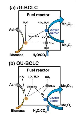
Fig. 6 Main reactions in the fuel reactor for solid fuels: (a) iG-BCLC (referred to as BCLC in this article) and (b) OU-BCLC
