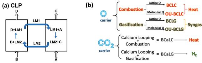
Fig. 4 (a) Schematic principles of chemical looping, and (b) classification basis for typical biomass-based CLPs.
