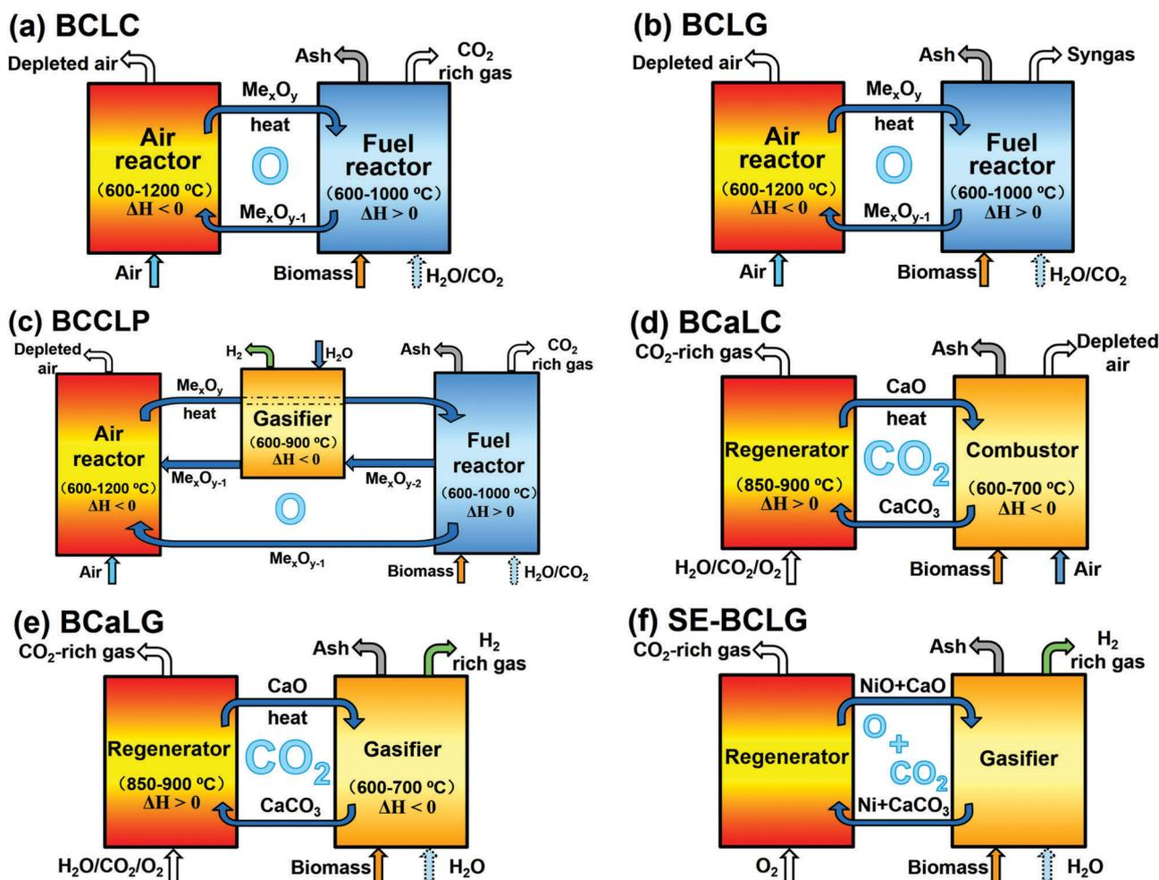
Fig. 5 Schematic principles of (a) biomass-based chemical looping combustion (BCLC), (b) biomass-based chemical looping gasification (BCLG), (c) biomass-based co-production chemical looping process (BCCLP), (d) biomass-based calcium looping combustion (BCaLC), (e) biomass-based calcium looping gasification (BCaLG) and (f) sorption-enhanced BCLG.
