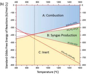
**Fig. 10** (a) Modified Ellingham diagram for oxygen carrier comparison and (b) zone of metal oxides for chemical looping. Reproduced from ref. 15 by permission from John Wiley & Sons Ltd.
