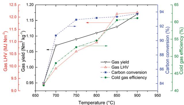
Fig. 9 Influence of temperature on the working properties of BCLG.<sup>71</sup>
