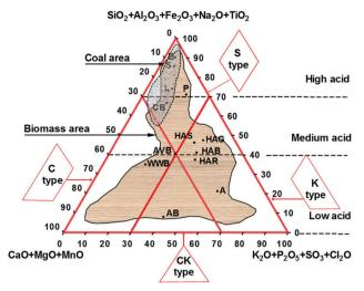
Fig. 3 Chemical classification of ashes and composition areas associated with biomass and coal ash. (Average values: A - algae, B - bituminous coal, S - sub-bituminous coal, L - lignite, P - peat, AB - animal biomass, CB - contaminated biomass, AVB - all varieties of biomass, HAB herbaceous and agricultural biomass, HAG – herbaceous and agricultural grass, HAS - herbaceous and agricultural straw, HAR - herbaceous and agricultural residue and WWB - wood and woody biomass.) Adapted from ref. 22.
