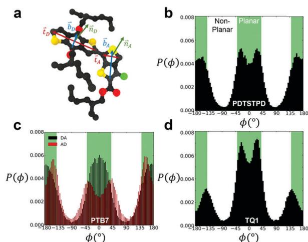
Fig. 2 Inter-ring dihedral distributions. (a) Diagram showing definitions of basis sets defining ring orientations for PTB7 monomer. Dihedral distributions,  $P(\phi)$ , obtained from simulations at 600 K and 1 atm for (b) PDTSTPD (c) PTB7 (d) TQ1. The *syn* conformations shown in Fig. 1 represent the planar arrangement that results from  $\phi = 0^\circ$ .
