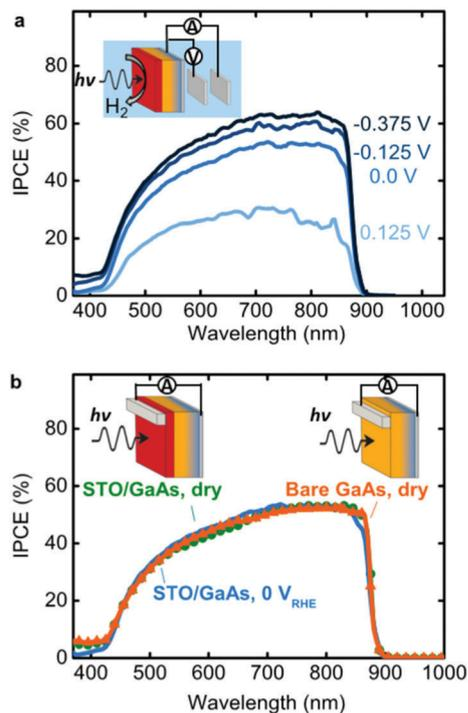
Fig. 3 Spectral response of SrTiO<sub>3</sub>/np-GaAs devices. (a) Incident photon-to-current efficiency (IPCE) in solution at different potentials near 0 V<sub>RHE</sub>. (b) IPCE of two-contact photovoltaic measurements with no electrolyte with and without SrTiO<sub>3</sub> compared to IPCE of photoelectrochemical HER at 0 V<sub>RHE</sub> (from panel a). Insets show schematics of measurement configurations.
