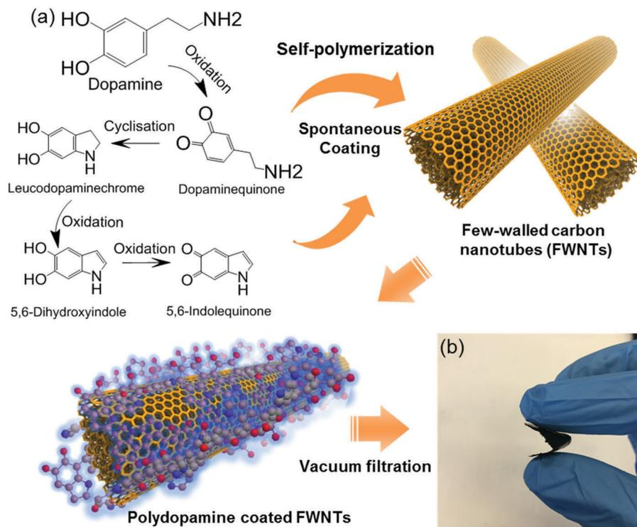
**Scheme 2** (a) Oxidative self-polymerization reactions of dopamine in weak alkaline solution and a continuous coating process of polydopamine on the surface of few-walled carbon nanotubes (FWNTs). (b) Digital image of a flexible hybrid film consisting of polydopamine coated FWNTs.
