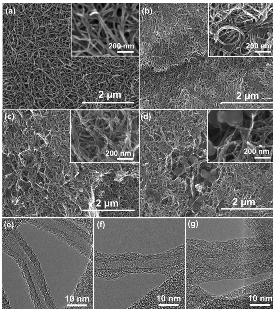
Fig. 4 Scanning electron microscopy (SEM) images of (a) the pristine FWNT and hybrid films: (b) PDA-2 (53 wt%), (c) PDA-4 (59.5 wt%), and (d) PDA-8 (65.6 wt%). The inset in (a–d) are the SEM images of FWNTs and hybrid films at high magnification. High resolution transmission electron microscopy (TEM) images of (e) pristine FWNT and hybrid films: (f) PDA-2 (39 wt%) and (g) PDA-2 (53 wt%).
