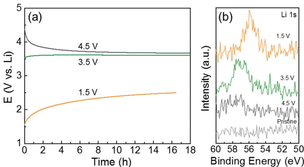
**Fig. 6** (a) The self-discharge course of the hybrid films after holding at different voltages. (b) XPS Li 1s spectra of the hybrid films (PDA-2, 53 wt%) after holding at different voltages and a continuous self-discharge test.
