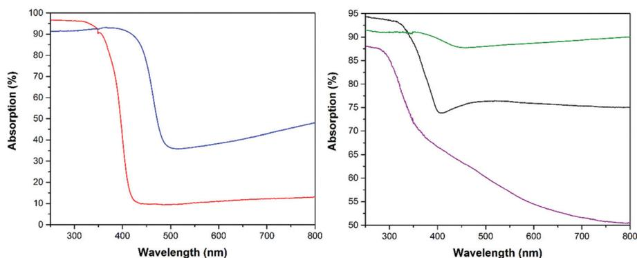
Fig. 3 Absorption spectra of the employed  $\text{WO}_3$  (blue) and  $\text{TiO}_2$  P25/20 (red) powders (left side) and of the cold sprayed  $\text{Ti}/\text{WO}_3$  (green) and  $\text{Ti}/\text{TiO}_2$  (black) photoelectrodes (right side). The purple curve on the right side shows the absorption spectra of the employed blank Ti substrate.
