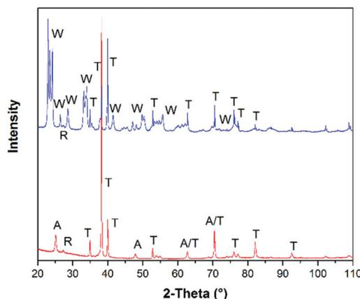
**Fig. 2** XRD patterns of WO<sub>3</sub> (blue) and TiO<sub>2</sub> (red) films deposited on titanium metal substrates by cold spray, where W denotes the WO<sub>3</sub> pattern, T the titanium metal pattern, R the rutile TiO<sub>2</sub> pattern and A the anatase TiO<sub>2</sub> pattern.
