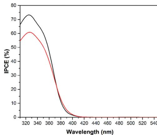
**Fig. 9** IPCE spectra for methanol oxidation measured for cold sprayed P25/20 on titanium metal (red) and screen printed P25 on FTO (black) photoanodes. Measurements for methanol oxidation were conducted in an aqueous solution of 0.5 M H<sub>2</sub>SO<sub>4</sub> with addition of 10 vol% of methanol (~2 mol L<sup>-1</sup>) at a bias of 1 V vs. NHE.
