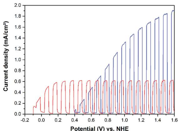
**Fig. 12** Chopped light current–potential curves of cold sprayed  $\text{WO}_3$  (blue) and  $\text{TiO}_2$  (red) on titanium metal photoanodes in 0.5 M  $\text{H}_2\text{SO}_4$  with addition of 10 vol% of methanol ( $\sim 2 \text{ mol L}^{-1}$ ). Measured with a scan rate of  $20 \text{ mV s}^{-1}$ . Current densities were measured upon irradiation with AM 1.5-global light (300 W Xe lamp).
