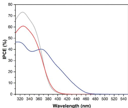
**Fig. 14** IPCE spectra for methanol oxidation employing cold sprayed  $\text{WO}_3$  (blue) and  $\text{TiO}_2$  (red) on titanium metal photoanodes. The IPCE curve of screen printed  $\text{TiO}_2$  on FTO photoelectrode is also given (light grey) for comparison. Measurements for methanol oxidation were conducted in an aqueous solution of 0.5 M  $\text{H}_2\text{SO}_4$  with addition of 10 vol% of methanol ( $\sim 2 \text{ mol L}^{-1}$ ) at a bias of 1 V vs. NHE.
