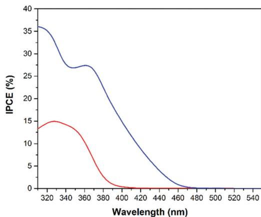
**Fig. 13** IPCE spectra for water oxidation employing cold sprayed  $\text{WO}_3$  (blue) and  $\text{TiO}_2$  (red) on titanium metal photoanodes. Measurements for water oxidation were conducted in an aqueous 0.5 M  $\text{H}_2\text{SO}_4$  solution at a bias of 1 V vs. NHE.
