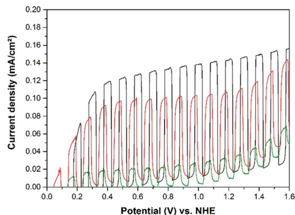
**Fig. 6** Chopped light current–potential curves of cold sprayed TiO<sub>2</sub> on titanium metal (red), screen printed TiO<sub>2</sub> on FTO (black) and screen printed TiO<sub>2</sub> on titanium metal (green) photoanodes in 0.5 M H<sub>2</sub>SO<sub>4</sub> recorded with a scan rate of 20 mV s<sup>−1</sup>. Current densities were measured upon irradiation with AM 1.5-global light (300 W Xe lamp).
