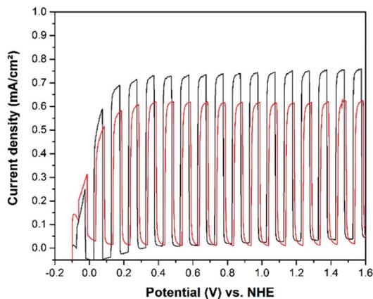
**Fig. 7** Chopped light current–potential curves of cold sprayed TiO<sub>2</sub> on titanium metal (red) and screen printed TiO<sub>2</sub> on FTO (black) photoanodes in 0.5 M H<sub>2</sub>SO<sub>4</sub> with addition of 10 vol% of methanol (~2 mol L<sup>-1</sup>). Measured with a scan rate of 20 mV s<sup>-1</sup>. Current densities were measured upon irradiation with AM 1.5-global light (300 W Xe lamp).
