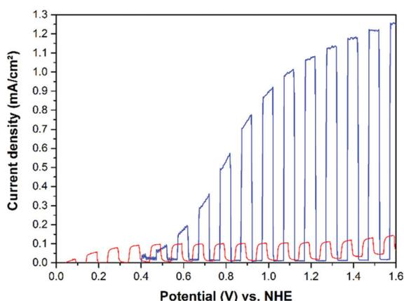
**Fig. 10** Chopped light current–potential curves of cold sprayed  $\text{WO}_3$  (blue) and  $\text{TiO}_2$  (red) on titanium metal photoanodes in 0.5 M  $\text{H}_2\text{SO}_4$  with a scan rate of  $20 \text{ mV s}^{-1}$ . Current densities were measured upon irradiation with AM 1.5-global light (300 W Xe lamp).
