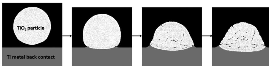
**Fig. 1** Scheme of the impact of a TiO<sub>2</sub> cold sprayed particle (white) on a Ti metal substrate (grey). The powder particle deforms and partially cracks during impact while the metal substrate deforms plastically. As a result, the TiO<sub>2</sub> particle is bonded to the metal without the help of any additive or binder.
