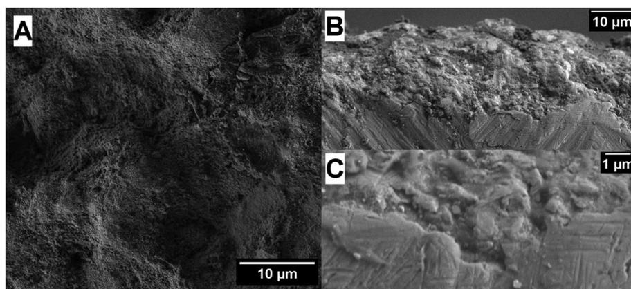
**Fig. 4** (A) SEM surface morphology image of a cold sprayed TiO<sub>2</sub> film. (B) Cross-sectional SEM image of a cold sprayed WO<sub>3</sub> film on a titanium substrate at a magnification of 1400 $\times$ . (C) Cross-sectional SEM image of the interface between the cold sprayed WO<sub>3</sub> film and the titanium substrate at a magnification of 8500 $\times$ .
