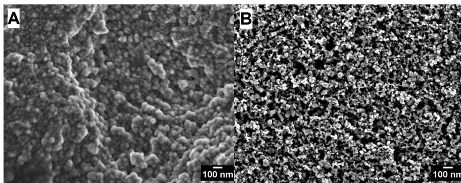
**Fig. 5** (A) SEM image of a cold sprayed TiO<sub>2</sub> (P25/20) film on Ti metal substrate. (B) SEM image of a screen printed TiO<sub>2</sub> (P25) film on FTO substrate.
