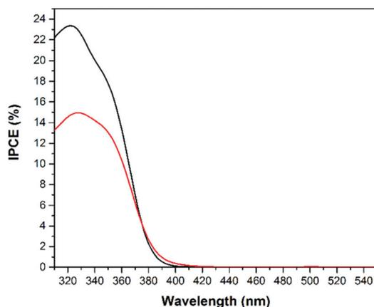
**Fig. 8** IPCE spectra for water oxidation measured for cold sprayed TiO<sub>2</sub> on titanium metal (red) and screen printed TiO<sub>2</sub> on FTO (black) photoanodes. Measurements for water oxidation were conducted in an aqueous 0.5 M H<sub>2</sub>SO<sub>4</sub> solution at a bias of 1 V vs. NHE.
