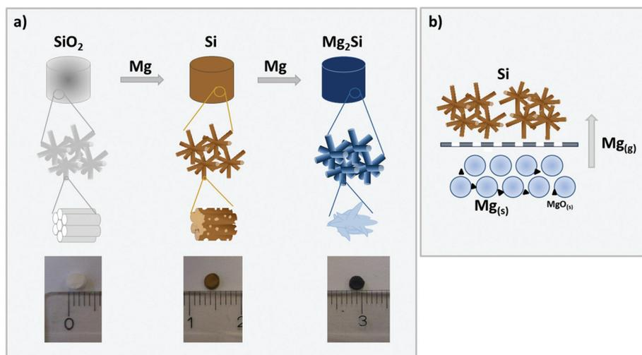
**Fig. 1** (a) Schematic illustration of the reduction of silica with magnesium vapor to give silicon in the first step and further reaction of silicon with Mg to yield Mg<sub>2</sub>Si; (b) reaction set-up in which the two precursors are spatially separated to avoid oxide impurities (MgO) in Mg<sub>2</sub>Si.
