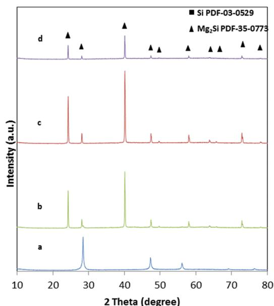
Fig. 5 XRD patterns of samples with different reaction temperatures (a) hierarchically structured porous silicon; (b) porous magnesium silicide  $600\text{ }^\circ\text{C} - 2\text{ h}$ ; (c) porous magnesium silicide  $650\text{ }^\circ\text{C} - 2\text{ h}$ ; (d) porous magnesium silicide  $700\text{ }^\circ\text{C} - 2\text{ h}$ .
