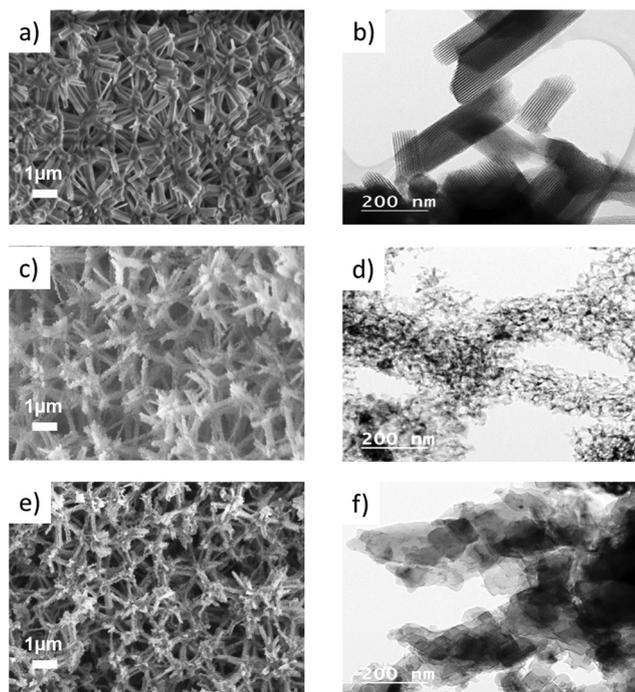
**Fig. 2** (a) SEM of cellular silica monolith; (b) TEM of mesoporous silica struts; (c) SEM of a cellular silicon network; (d) TEM of aggregated silicon nanocrystallites; (e) SEM of a magnesium silicide cellular network; (f) TEM of magnesium silicide crystallites forming the struts in the cellular network.
