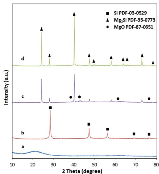
**Fig. 3** XRD patterns of (a) hierarchically structured macro/mesoporous amorphous silica; (b) hierarchically structured porous silicon 650 °C – 2 h; (c) porous magnesium silicide with MgO as impurity while mixing the precursors 650 °C – 30 min; (d) porous magnesium silicide from the reaction set-up with spatially separated precursors 650 °C – 30 min.
