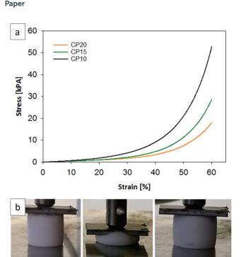
Fig. 3 (a) Stress-strain curves of the chloropropyl functionalized gels (CP10, CP15 and CP20), (b) uniaxial compression test (60% of the original height) on a CP10 sample showing reversible compression.
