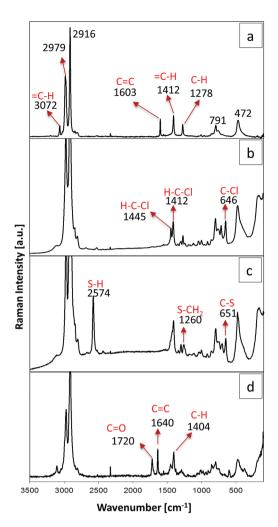
Fig. 4 Raman spectra of the samples (a) V20, (b) CP20, (c) MP20 and (d) MAP20.
