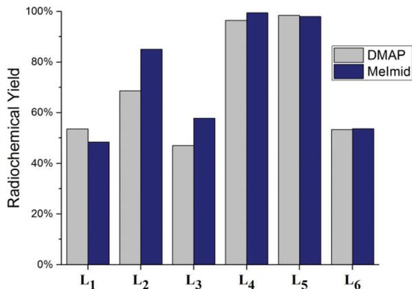
Fig. 5 Radiochemical labeling yields of the reaction of with monodentate ligands DMAP (gray) and Melmid (blue) with  $fac-[^{99m}Tc(CO)_3(L)(OH_2)]^{0/+}$  containing bidentate ligands (L<sub>1</sub>–L<sub>6</sub>) to yield the respective product  $fac-[^{99m}Tc(CO)_3(L)(DMAP/Melmid)]^{0/+}$ .
