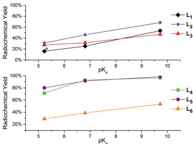
**Fig. 4** Plot of radiochemical yields of 2 + 1 formation with monodentate pyridine ligands (a–c) vs. pK<sub>a</sub> of monodentate pyridine ligands. Neutral bidentate ligands (L<sub>1–3</sub>) (top), anionic bidentate ligands (L<sub>4–6</sub>) (bottom) and pyridine ligands (py (pK<sub>a</sub> 5.33), 4-MP (pK<sub>a</sub> 6.55), DMAP (pK<sub>a</sub> 9.71)). \*Yield for 1a' estimated at 16% for this plot due to peak overlap.
