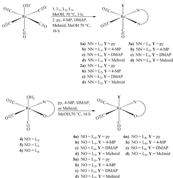
**Scheme 1** Synthesis of 2 + 1 complexes,  $fac-[Re^I(CO)_3(L)(Y)]^{0/+}$ , with bidentate ligands (**L**<sub>1</sub>–**L**<sub>6</sub>) and monodentate aromatic amine ligands (**Y**). Top: a two-step one pot procedure for neutral ligands (**L**<sub>1</sub>–**L**<sub>3</sub>) and **Y**. Bottom: second step using the intermediate  $fac-[Re^I(CO)_3(L)(OH_2)]$  of anionic ligands (**L**<sub>4</sub>–**L**<sub>6</sub>) with **Y**.
