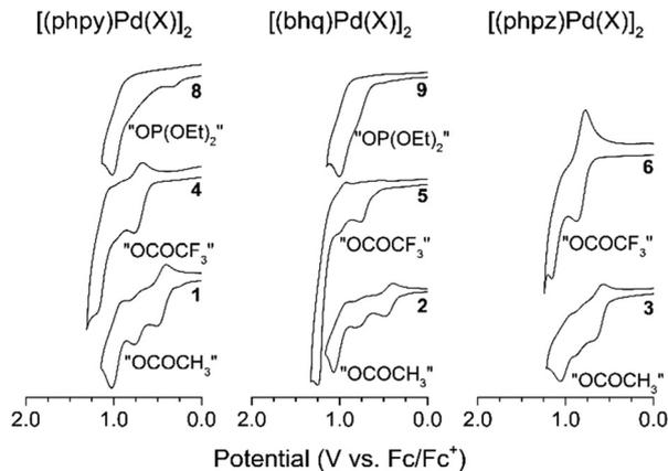
Fig. 6 Cyclic voltammograms of palladacycles in  $\text{CH}_2\text{Cl}_2$ .
