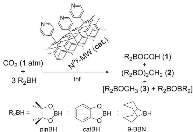
**Scheme 1**  $CO_2$  reduction catalyzed by  $N^{Py}$ -MW with various hydroboranes and the distribution of products (1–3). See also Fig. 1.
