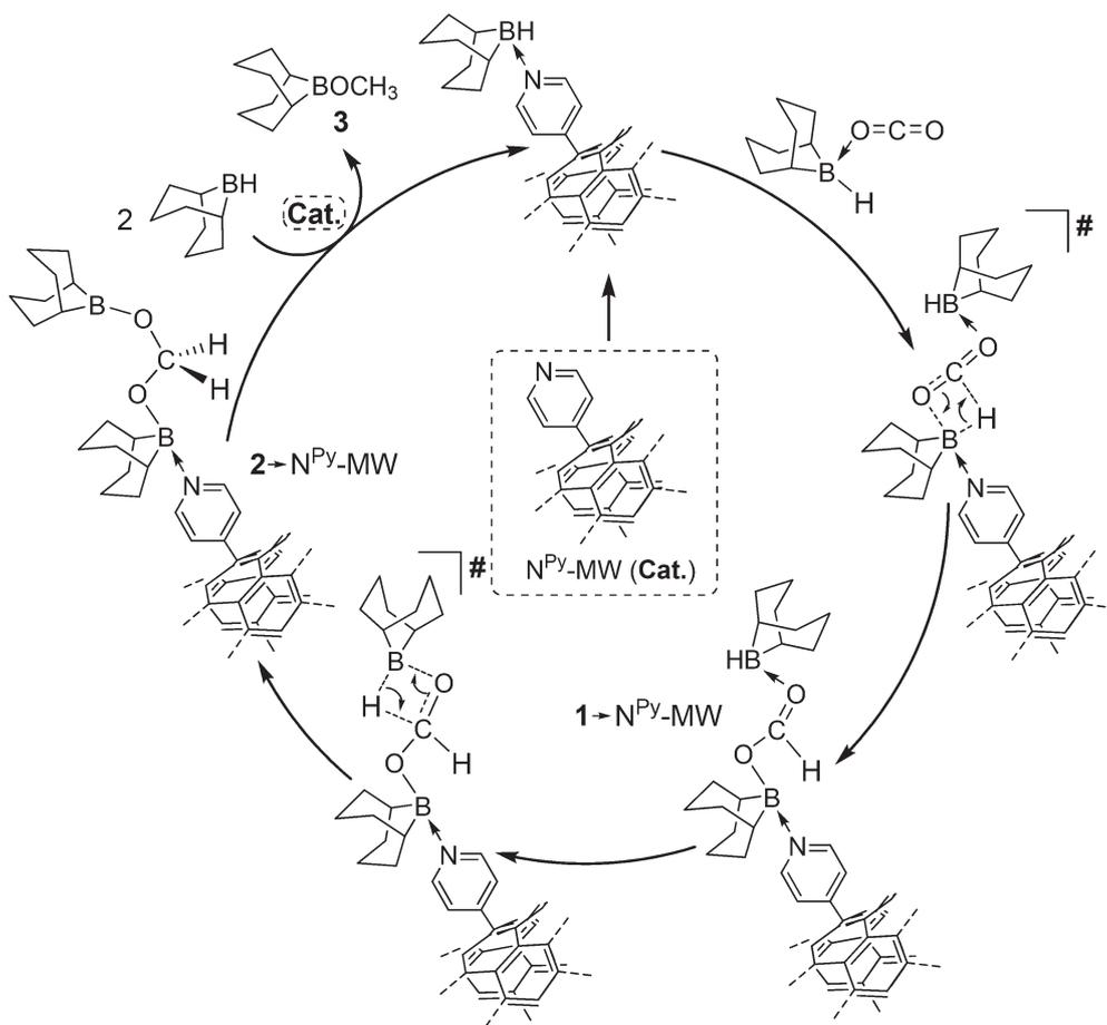
**Scheme 2** Proposed mechanism for the CO<sub>2</sub> reduction catalyzed by N<sup>Py</sup>-MW in the presence of 9-BBN. See the ESI† for details on DFT calculations related to the postulated reaction path.
