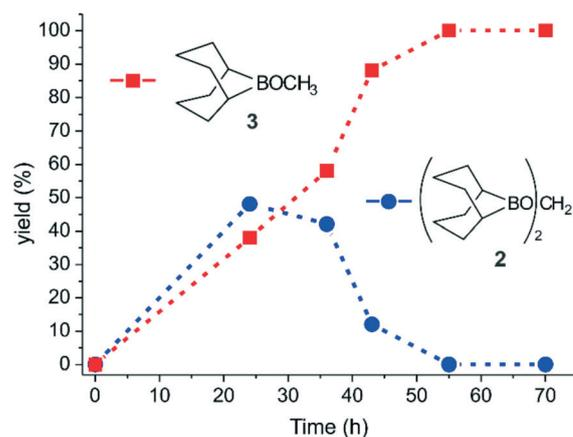
**Fig. 1** Product distribution (%) over time (h) for the catalytic reduction of  $CO_2$  (1 bar) with  $N^{Py}$ -MW as the catalyst and 9-BBN as the reducing agent. Yields (%) of 2 and 3 are from entries 1–4 of Table 2.
