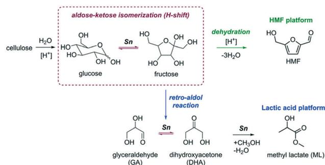
Fig. 1 Reaction pathways for the catalytic conversion of cellulose into the renewable chemical platform molecules 5-hydroxymethylfurfural (HMF) and lactic acid. The role of Lewis acid Sn and Brønsted acid sites is indicated.
