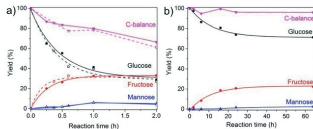
**Fig. 7** The evolution of the composition of the reaction mixtures with time for glucose isomerization over a) Sn-Beta and b) Sn-MOR-bulk. Conditions: a) 2.5 mL of 125 mM glucose in water, 100 °C; b) 2.5 mL of 125 mM glucose in water, 100 °C, 40 mg cat. Dashed lines, open symbols (a): Sn-Beta-nano, solid lines, closed symbols: [Sn]-Beta-HF.
