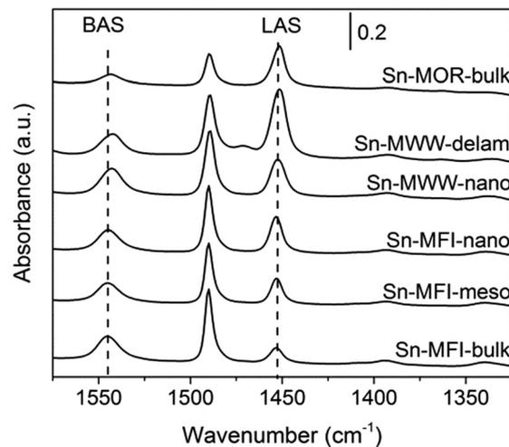
Fig. 5 FTIR spectra of adsorbed pyridine on selected Sn-containing zeolite catalysts. Absorption bands due to pyridine interacting with Brønsted and Lewis acid sites are indicated as BAS and LAS, respectively.
