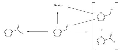
Fig. 3 Proposed reaction pathways operational when furfural is oxidised over AuPd/Mg(OH)<sub>2</sub> under basic conditions.
