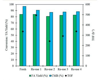
Fig. 5 A re-use study for the oxidation of FF over fresh and used samples of the 1 wt%  $AuPd/Mg(OH)_2$  catalyst. The FA yield and CMB data reflects samples taken after of 4 h of reaction. The TOF is assessed after 0.5 h. Reaction conditions: 303 K, p: 3 bar  $O_2$ , NaOH: FF equivalents: 1, reaction volume (10 mL), catalyst (91.1 mg).
