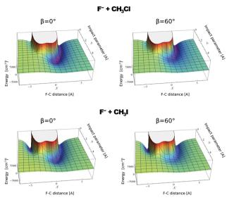
Fig. 10 Computed potential energy for F<sup>-</sup> approaching CH<sub>3</sub>Cl (up) and CH<sub>3</sub>I (low) as a function of impact parameter (b) and F-C distance. The two values of  $\beta$  represent the two possible dihedral angles between the C, Y, H and X atoms. The potentials are reproduced with permission from ref. 159.
