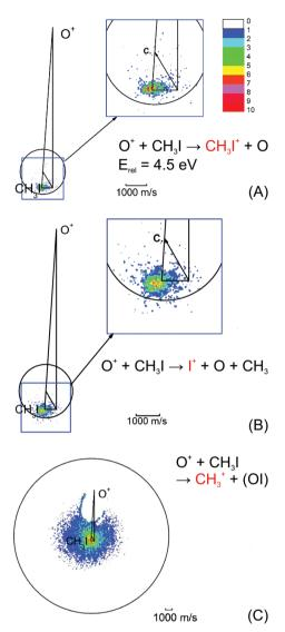
Fig. 4 Velocity map images for all three possible product channels in the reaction  $CH_3I + O^+$ : (A)  $CH_3I^+$ , (B)  $I^+$  and (C)  $CH_3^+$ . The formation of  $CH_3^+$  is the dominant product channel in the reaction with CH<sub>3</sub>I (65%). The charge transfer product CH<sub>3</sub>I<sup>+</sup> is the least abundant (15%). The circle indicates the maximum ion velocity considering energy and momentum conservation. Reprinted with permission from ref. 96.
