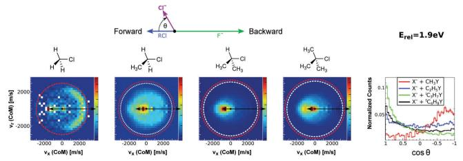
Fig. 15 Center-of-mass velocity distribution and scattering angle of product  $Cl^-$  ions produced in the reactions (from left to right)  $F^- + CH_3Cl$ ,  $F^- + C_2H_5Cl$ ,  $F^- + iC_3H_7Cl$  and  $F^- + iC_4H_9Cl$ . The kinematical limits for the  $S_N2$  and  $EC_N2$  and  $EC_$
