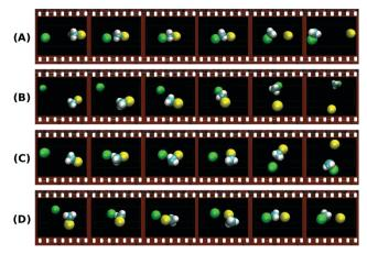
Fig. 8 Exemplary trajectories along the reaction coordinate of a typical  $S_N 2$  reaction showing some of the major atomistic mechanisms found in the theoretical simulations:  $^{144,153}$  (A) direct backward; (B) forward stripping; (C) indirect; (D) roundabout. The full animations of the trajectories can be found at http://hase-group.ttu.edu/animations.html.
