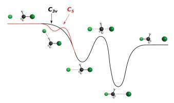
Fig. 7 Schematic representation of a typical minimal energy path for the collinear ( $C_{3v}$ ) and X-H bonded ( $C_s$ ) nucleophilic substitution reaction. The optimized chemical structures shown for the most important stationary points have been taken from ref. 143
