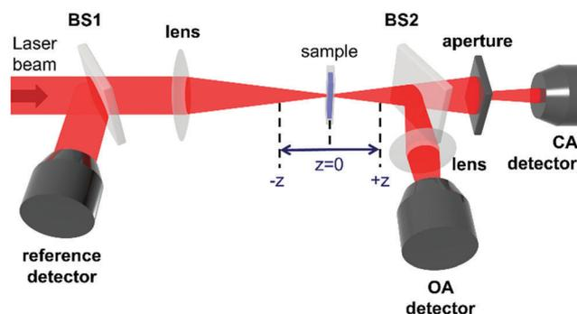
Fig. 2 The representation of a typical Z-scan setup.
