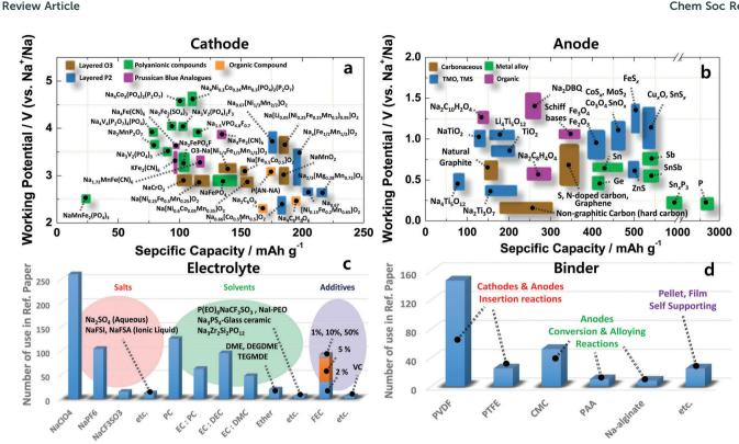
Fig. 1 Recent research progress in sodium ion batteries: (a) cathode, (b) anode, (c) electrolyte and (d) binder.
