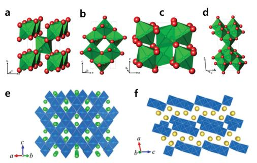
Fig. 24 Crystal structures of TiO<sub>2</sub>. (a) Rutile, (b) anatase, (c) bronze, (d) brookite. (Reprinted from ref. 299, Copyright 2015, with permission from Elsevier.) Crystal structures of (e) spinel-type Li<sub>4</sub>Ti<sub>5</sub>O<sub>12</sub> and (f) Na<sub>2</sub>Ti<sub>3</sub>O<sub>7</sub>. Li and Na atoms are represented by green and yellow spheres, respectively. (Reproduced with permission from ref. 300, Copyright 2016 The Royal Society of Chemistry.)
