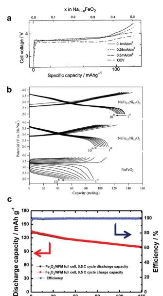
Fig. 3 (a) Charge and discharge curves of O3-NaFeO2. (Reprinted from ref. 39, Copyright 1994, with permission from Elsevier.) (b) Charge and discharge curves of O3-Na[Fe<sub>1-x</sub>Ni<sub>x</sub>]O<sub>2</sub>. (Reproduced with permission from ref. 48, Copyright 2014 American Chemical Society.) (c) Clce performance for the  $Fe_3O_4/Na[Ni_{0.25}Fe_{0.5}Mn_{0.25}]O_2$  full cell. (Reproduced with permission from ref. 51, Copyright 2014 American Chemical Society.)
