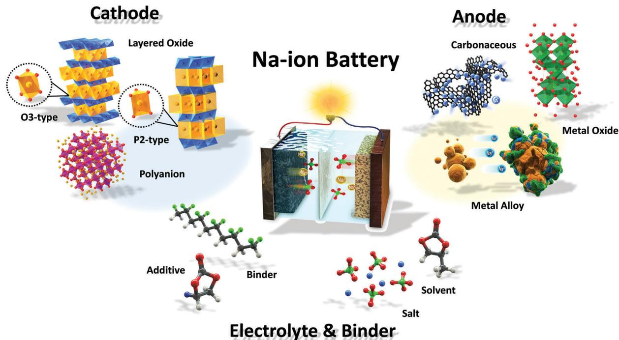
Scheme 1 Illustration of a Na-ion battery system.
