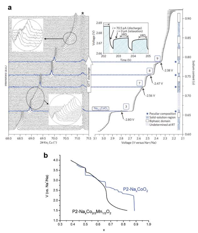
Fig. 6 (a) In situ XRD patterns during sodium ion intercalation in P2-Na<sub>x</sub>CoO<sub>2</sub>. (Reproduced by permission from ref. 62, Nature Publishing Group, Copyright 2011.) (b) Comparison between the second discharges obtained for a P2-Na<sub>x</sub>[Co<sub>2/3</sub>Mn<sub>1/3</sub>]O<sub>2</sub> cell (black curve) and a Na<sub>x</sub>CoO<sub>2</sub> cell (blue curve). (Reproduced with permission from ref. 76, Copyright 2011 The Royal Society of Chemistry.)
