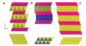
Fig. 2 Crystal structures; (a) perspective view (top) and top view of the (001) layer of the O3 structure, (b) perspective view (top) and top view of the (001) layer of the P2 structure in which yellow sphere is face shared Na1 and blue one is edge sharing Na2 atoms, and (c) perspective view (top) and top view of the (001) layer of the P3 structure.
