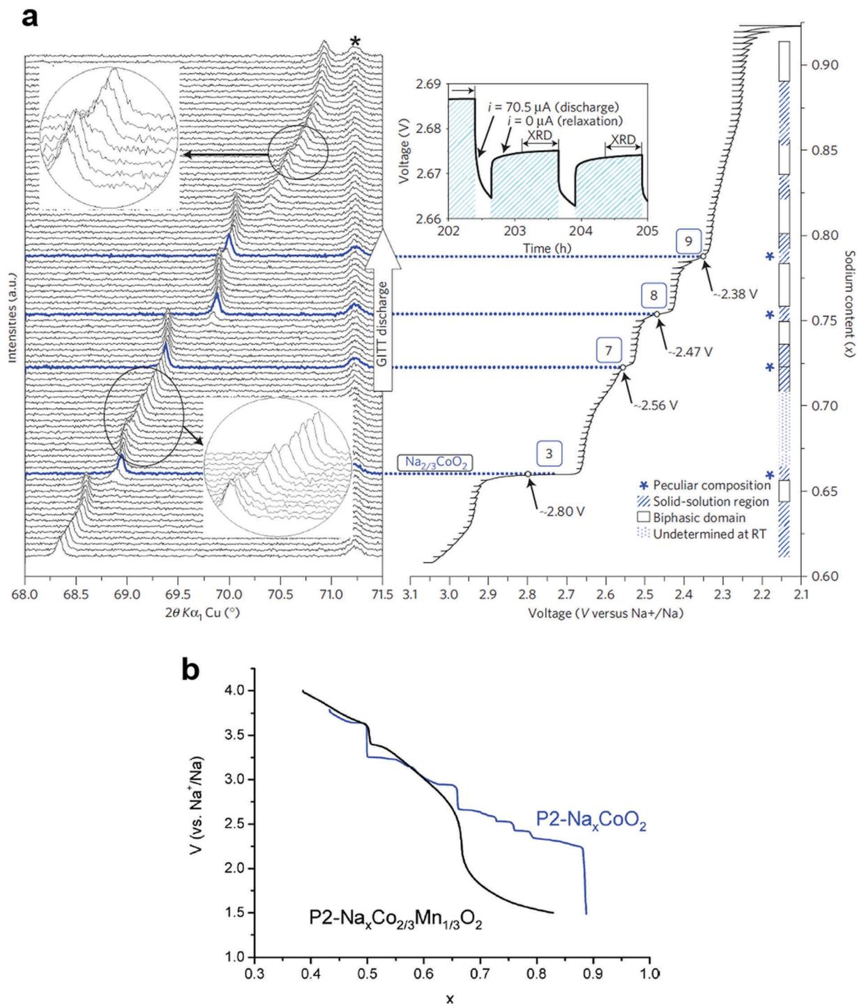
Fig. 6 (a) *In situ* XRD patterns during sodium ion intercalation in P2- $\text{Na}_x\text{CoO}_2$ . (Reproduced by permission from ref. 62, Nature Publishing Group, Copyright 2011.) (b) Comparison between the second discharges obtained for a P2- $\text{Na}_x[\text{Co}_{2/3}\text{Mn}_{1/3}]\text{O}_2$  cell (black curve) and a  $\text{Na}_x\text{CoO}_2$  cell (blue curve). (Reproduced with permission from ref. 76, Copyright 2011 The Royal Society of Chemistry.)
