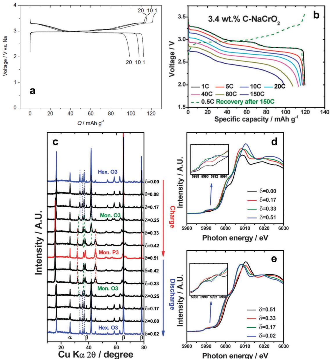
Fig. 10 (a) Charge and discharge curves of O3-NaCrO<sub>2</sub>. (Reprinted from ref. 128, Copyright 2010, with permission from Elsevier.) (b) Rate performances of 3.4 wt% carbon-coated O3-NaCrO<sub>2</sub>. (c) *Ex situ* XRD patterns obtained during charging and discharging, Cr K-edge XANES spectra obtained during (d) charging and (e) discharging. (Reproduced with permission from ref. 130, Copyright 2015 The Royal Society of Chemistry.)
