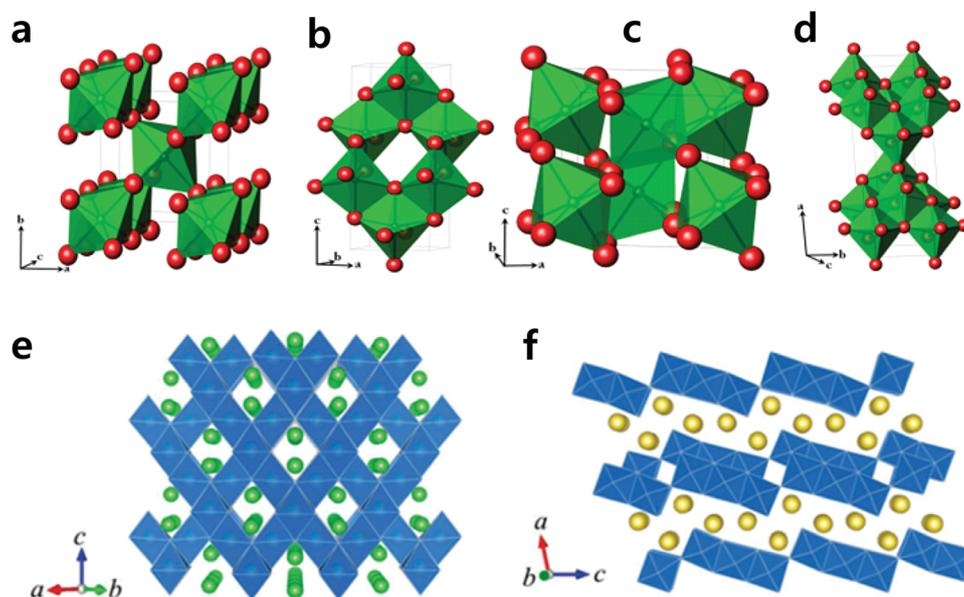
Fig. 24 Crystal structures of TiO<sub>2</sub>. (a) Rutile, (b) anatase, (c) bronze, (d) brookite. (Reprinted from ref. 299, Copyright 2015, with permission from Elsevier.) Crystal structures of (e) spinel-type Li<sub>4</sub>Ti<sub>5</sub>O<sub>12</sub> and (f) Na<sub>2</sub>Ti<sub>3</sub>O<sub>7</sub>. Li and Na atoms are represented by green and yellow spheres, respectively. (Reproduced with permission from ref. 300, Copyright 2016 The Royal Society of Chemistry.)
