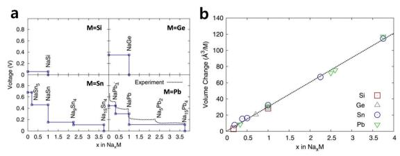
Fig. 34 (a) Na-M voltage curves calculated using DFT and (b) the volume changes for group 14 elements in periodic table. (M = Si, Ge, Sn, and Pb.) Experimental values are also given if available. (Reproduced with permission from ref. 244, Copyright 2011 The Electrochemical Society.)
