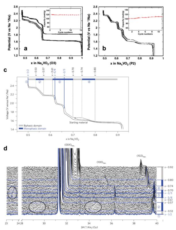
Fig. 11 Voltage-composition curves of (a) O3-NaVO2 and (b) P2-Na<sub>0.7</sub>VO2. (Reprinted from ref. 135, Copyright 2011, with permission from Elsevier.) P2-Na<sub>x</sub>VO<sub>2</sub>: (c) the limits of the biphasic domains and the solid solutions (d) in situ X-ray diffraction data recorded during the galvanostatic intermittent titration technique experiments. (Reproduced by permission from ref. 136, Nature Publishing Group, Copyright 2013.)
