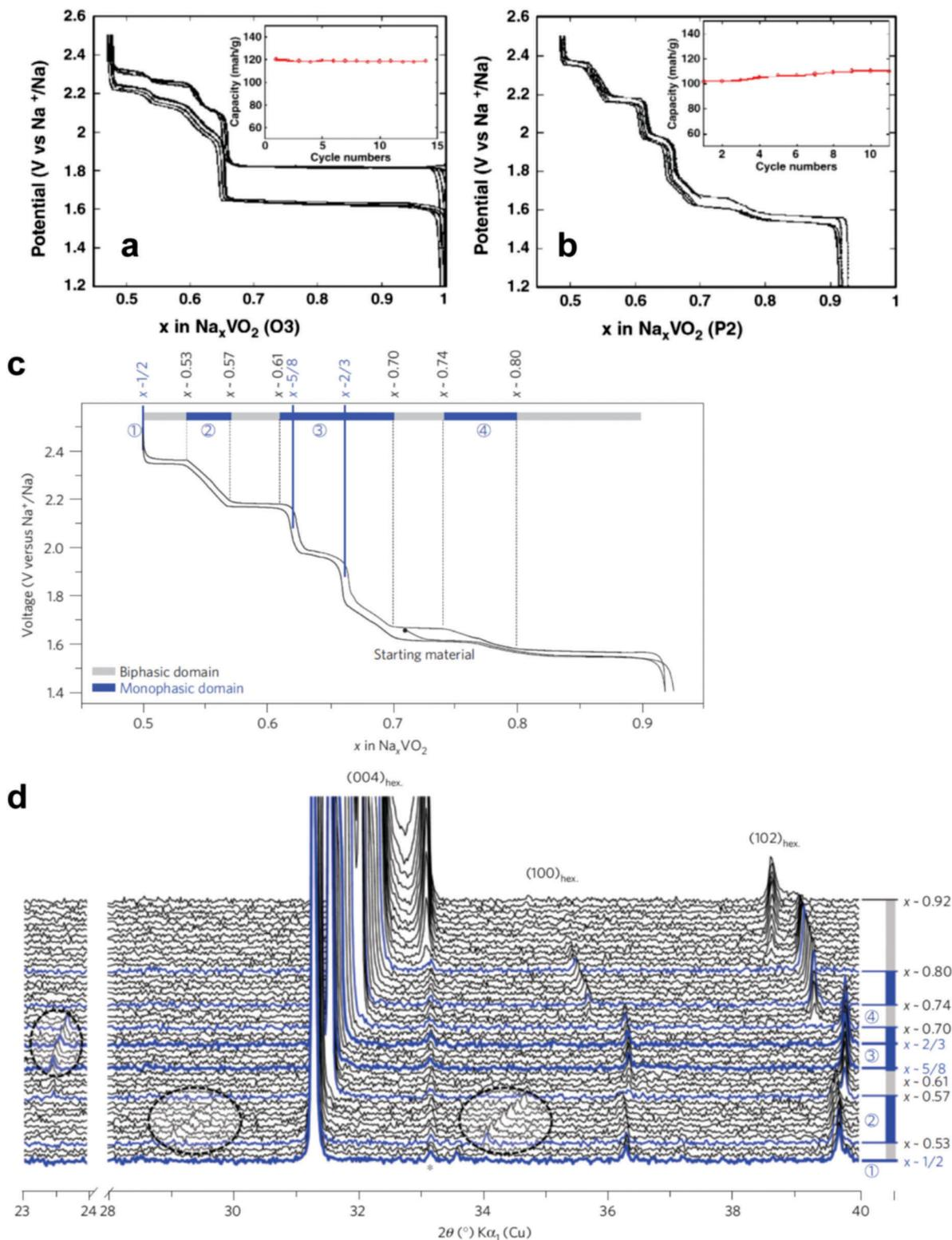
**Fig. 11** Voltage–composition curves of (a) O3- $\text{NaVO}_2$  and (b) P2- $\text{Na}_{0.7}\text{VO}_2$ . (Reprinted from ref. 135, Copyright 2011, with permission from Elsevier.) P2- $\text{Na}_x\text{VO}_2$ ; (c) the limits of the biphasic domains and the solid solutions (d) *in situ* X-ray diffraction data recorded during the galvanostatic intermittent titration technique experiments. (Reproduced by permission from ref. 136, Nature Publishing Group, Copyright 2013.)
