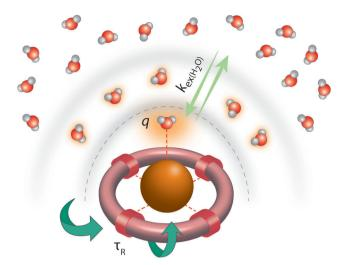
Fig. 3 In activatable,  $T_1$ -weighted MRI contrast agents, MR signal change can be generated via modulation of the main parameters that determine relaxivity: the number of water molecules directly coordinated to the paramagnetic ion (Gd $^{3+}$ ), q; the exchange rate of the inner sphere water with bulk water,  $k_{\text{ex}(\text{H}_2\text{O})}$ ; the rotational motion of the complex, characterized by the rotational correlation time,  $\tau_{\rm R}$ .
