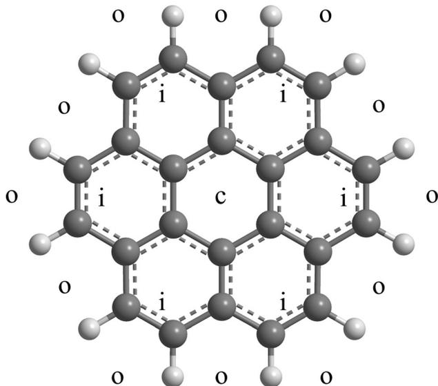
Fig. 1 Approximate location of the central (c), inner (i) and outer (o) adsorption sites on one face of  $(\text{H}_2)_{38}\text{Cor}^+$ .
