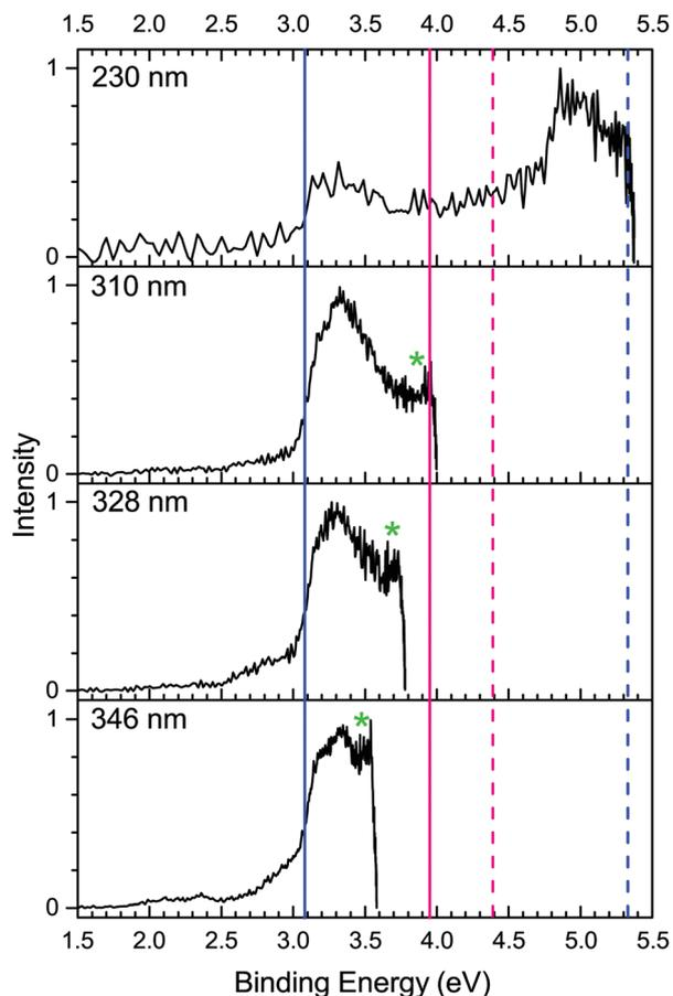
Fig. 4 Gas-phase photoelectron spectra of  $iLH^-$  deprotonated anions produced by electrospray ionisation from 1 mM dry methanol solution. Vertical blue and pink lines mark the EOM-IP-CCSD calculated vertical detachment energies of the phenolate and carboxylate isomers, respectively ( $D_0$  = solid,  $D_1$  = dashed). The asterisks indicate the broadening to the high binding energy side of the direct detachment feature (see text).
