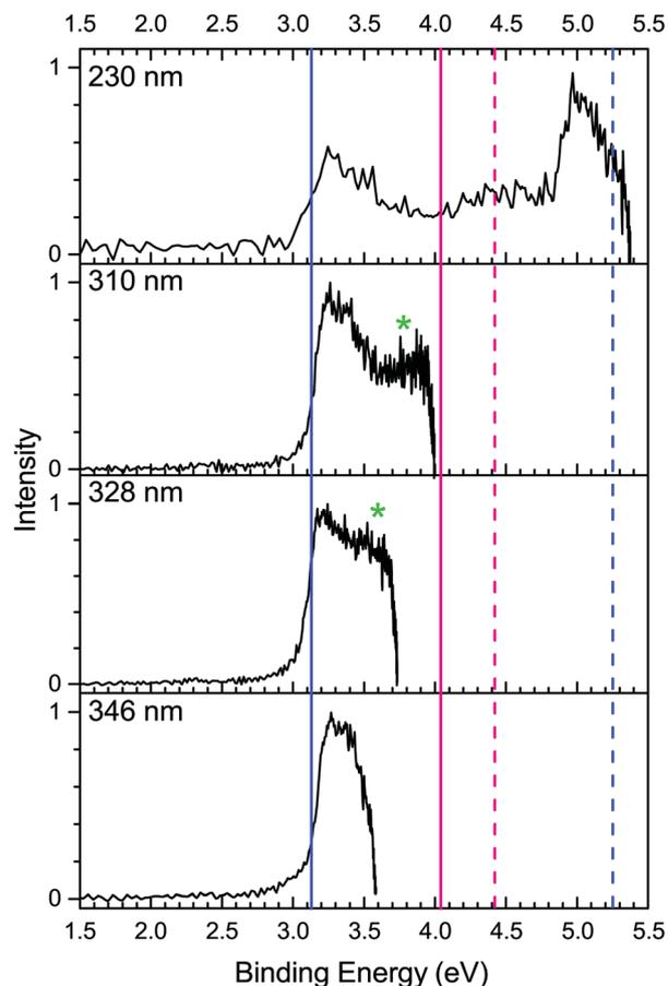
Fig. 3 Gas-phase photoelectron spectra of  $\text{LH}^-$  deprotonated anions produced by electrospray ionisation from 1 mM dry methanol solution. Vertical blue and pink lines mark the EOM-IP-CCSD calculated vertical detachment energies of the phenolate and carboxylate isomers, respectively ( $D_0$  = solid,  $D_1$  = dashed). The asterisks indicate the broadening to the high binding energy side of the direct detachment feature (see text).
