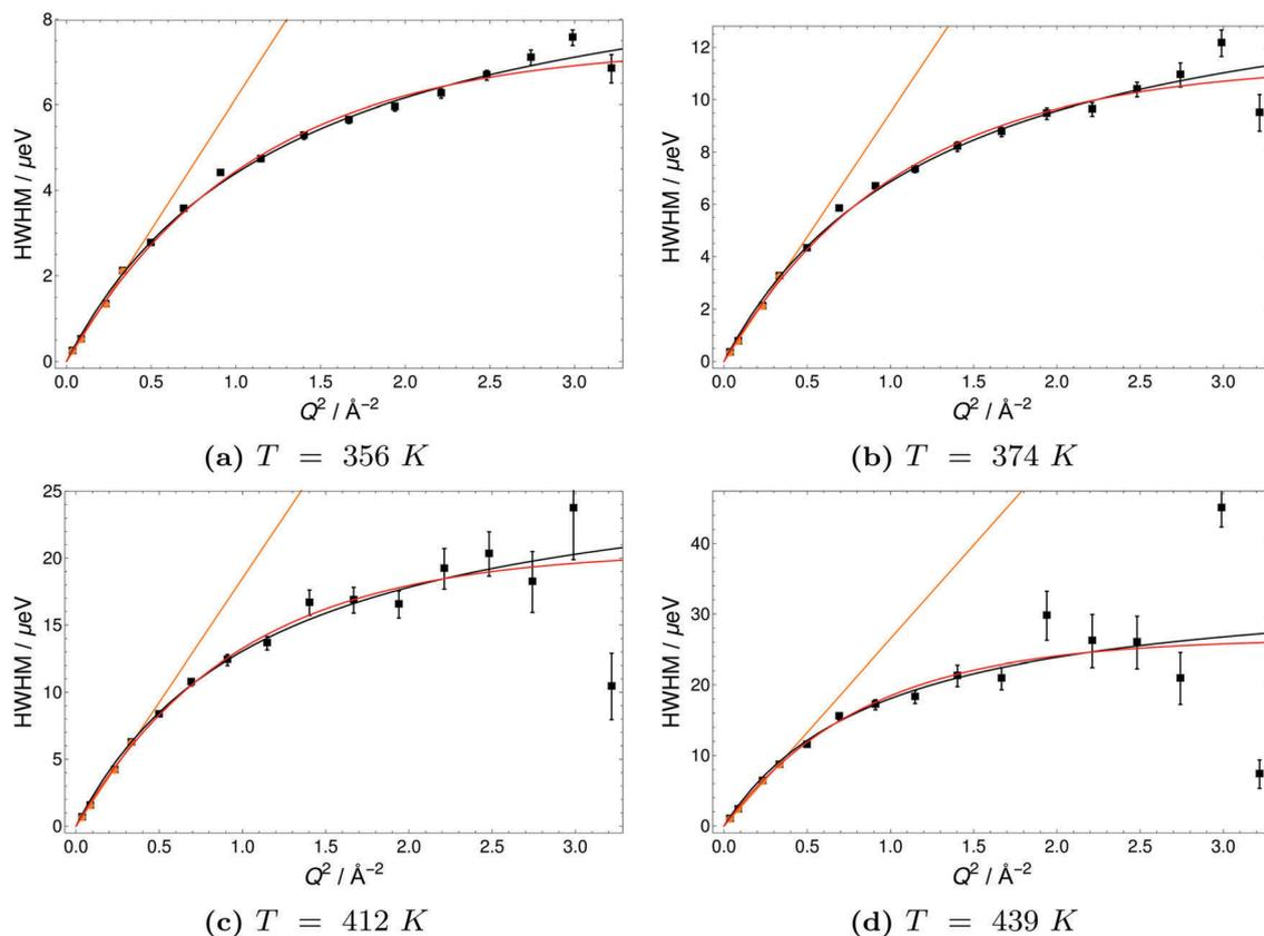
Fig. 10 Half-Width-at-Half-Maximum (HWHM) of quasielastic scattering peaks of 6PA1BI versus momentum transfer  $Q^2$  at different temperatures. Orange lines indicate a fit of the  $DQ^2$ , black lines a Singwi-Sjölander model (SS) fit and red lines a Hall-Ross (HR) fit.
