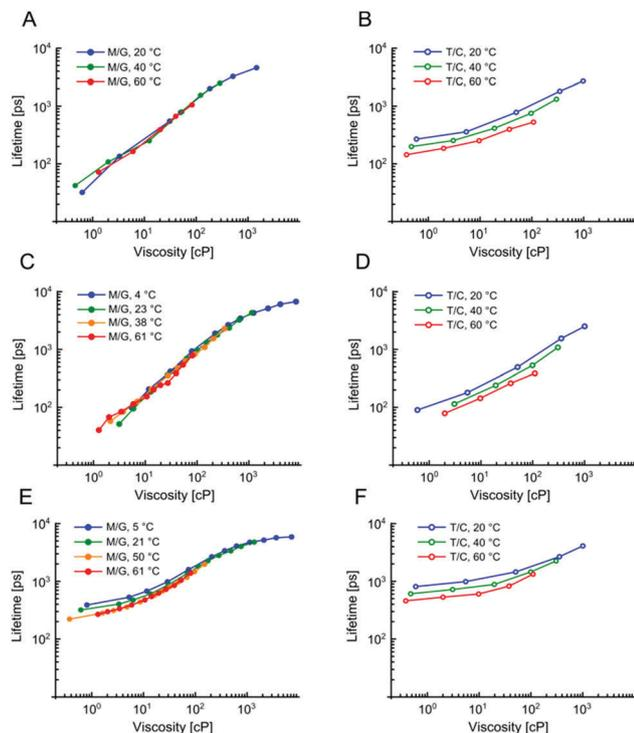
Fig. 2 The fluorescence lifetimes of **2** (A and B), **3** (C and D) and **1** (E and F) at different viscosities, temperatures and solvent polarities. The fluorescence lifetimes were measured in methanol–glycerol (A, C and E) and castor–toluene (B, D and F) mixtures. The results demonstrate that the dyes are affected not only by viscosity but by temperature and polarity as well.
