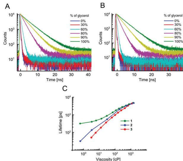
Fig. 1 The fluorescence decays of **2** (A) and **3** (B) in methanol–glycerol mixtures at 20 °C. (C) The fluorescence lifetimes of **2** (blue) and **3** (red) in methanol glycerol mixtures in comparison with the lifetimes of the previously reported molecular rotor **1**. Excitation and emission wavelengths were 480 nm and 520 nm, respectively.
